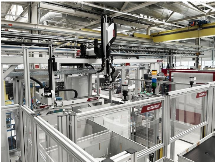
Two WITTMANN linear robots ensure a smooth and efficient process.
