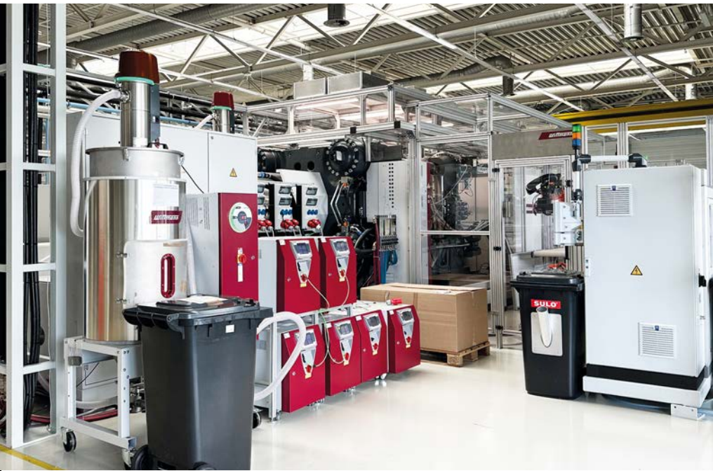
The Tempro plus D temperature controllers contribute to short cycle times thanks to their high cooling performance.
