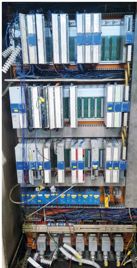
The control cabinet of a large injection molding machine built in 1989 before (left) and after the integration (right) of a Unilog B8 control system. The new control system components require considerably less space. This leaves room for additional options without taking up any extra production floor space.
