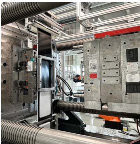
The individual picture frames are fed into the mold cavity while demolding the finished injection-molded part.
