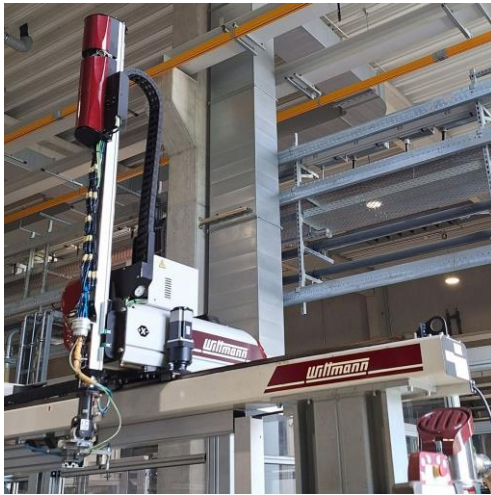
Linear robots from WITTMANN play a vital part in the standardized automation cells at Rauschert.
