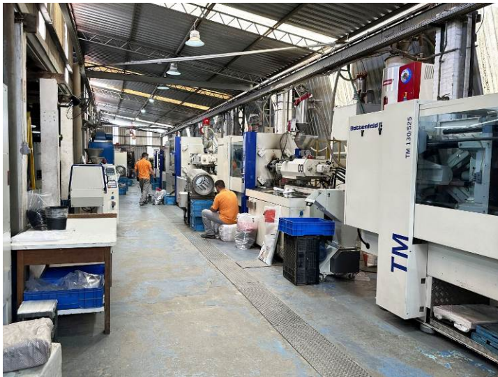
Fig. 10: The equipment in the injection molding hall consists of 16 machines. The company's first DC machine will be started up shortly.
