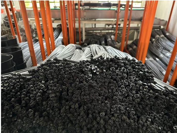
Fig. 4: Plasnova operates several extrusion lines for making pipes and hoses.
