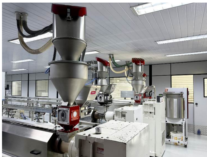
Fig. 7: All extrusion lines, too, are equipped exclusively with material loaders, dryers and dosing systems from WITTMANN.
