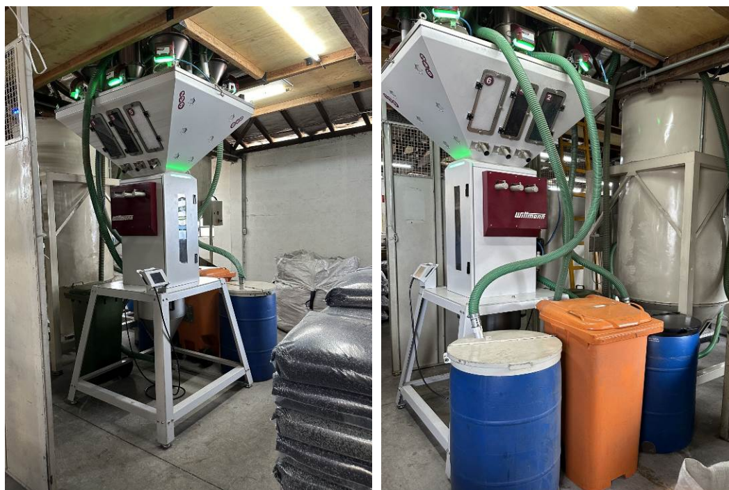
Fig. 6a+b: The new large Gravimax meters and mixes together up to six materials with extreme precision.
