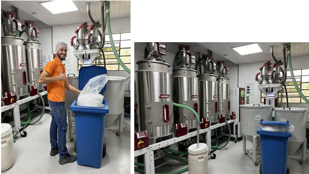
Fig. 8a+b: The central materials handling system makes it easier for staff members to manufacture products with highest possible material efficiency and process consistency.
