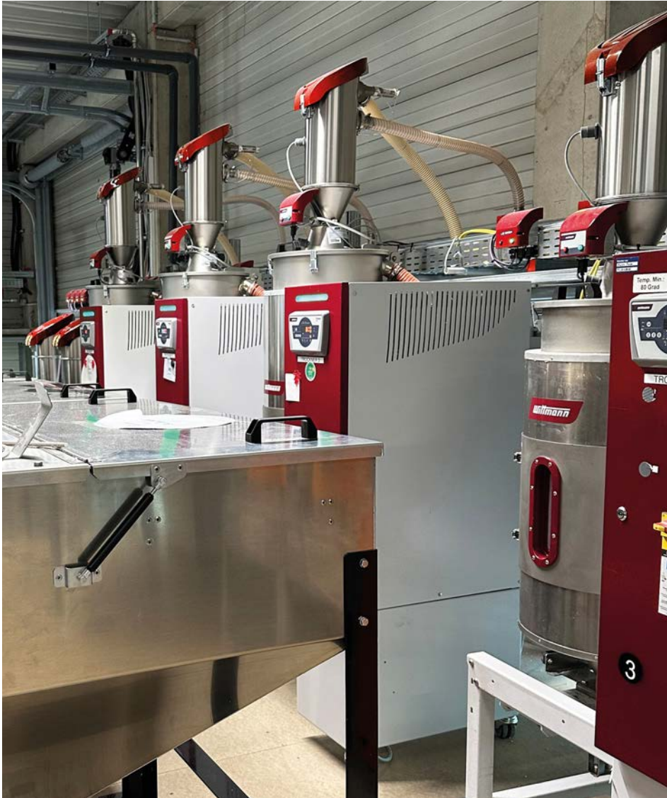
The Central Material Supply System includes Drymax material dryers.
