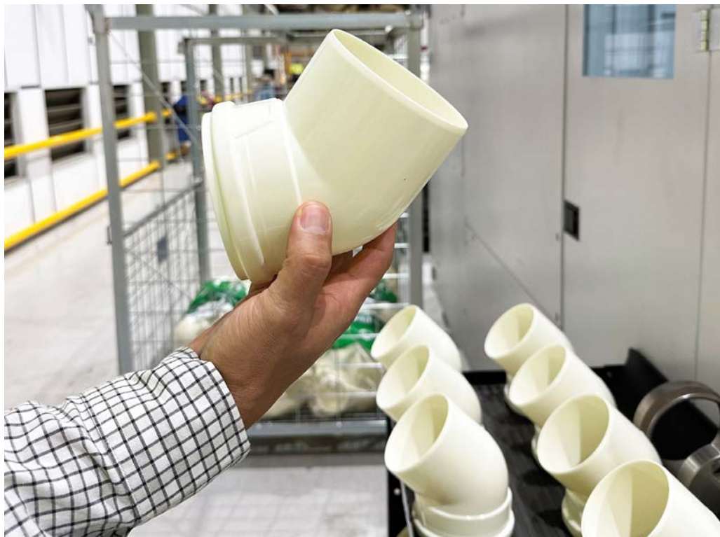
Pipe elbows produced efficiently: Amanco Wavin invested in a new injection molding department to strengthen the local facilities in Brazil.
