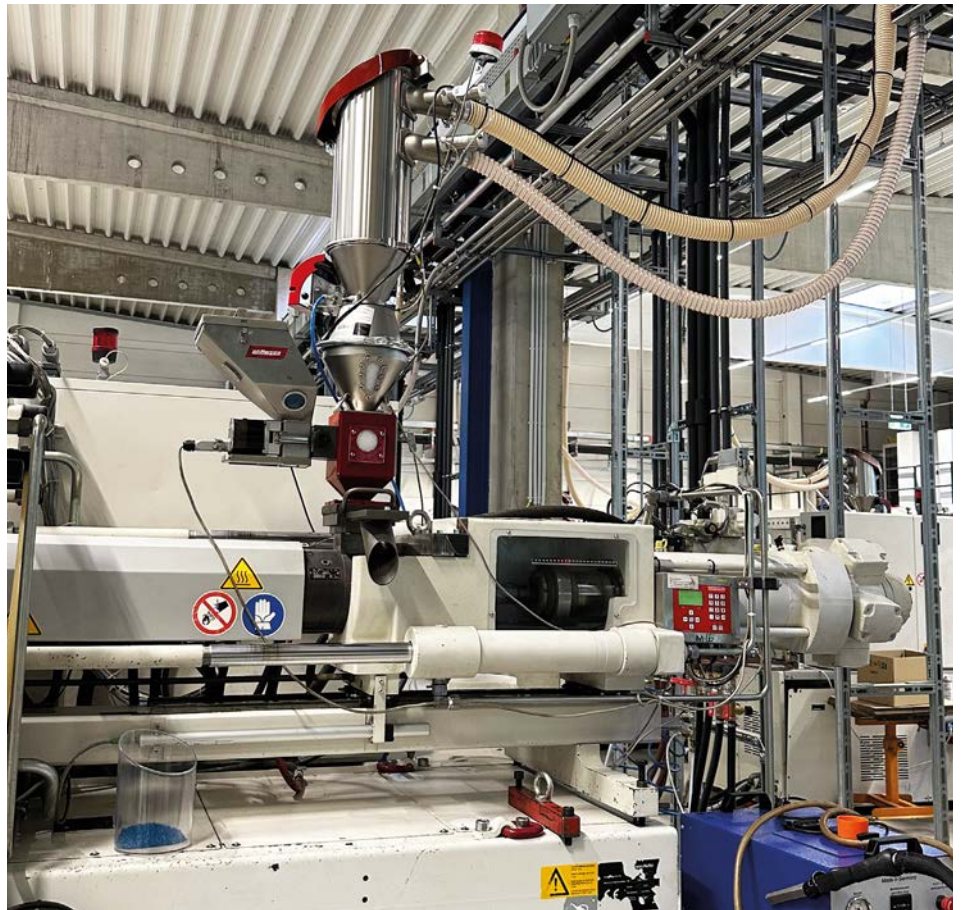
The granulate is transported inside a closed system. Feedmax Clean material loaders are also used. In this way, dust generation is reliably prevented.
