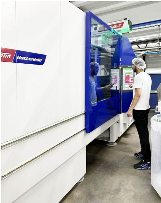
Fig. 4a+b: The control system integration of both the injection molding machine and the robot facilitates operation of the production cell.
