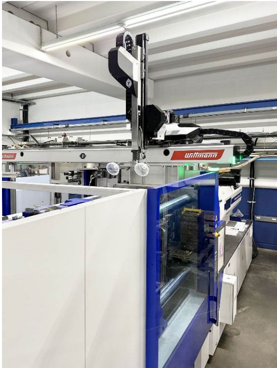
Fig. 3: The Sonic high-speed robot has been specially developed for high-speed applications in the packaging industry.
