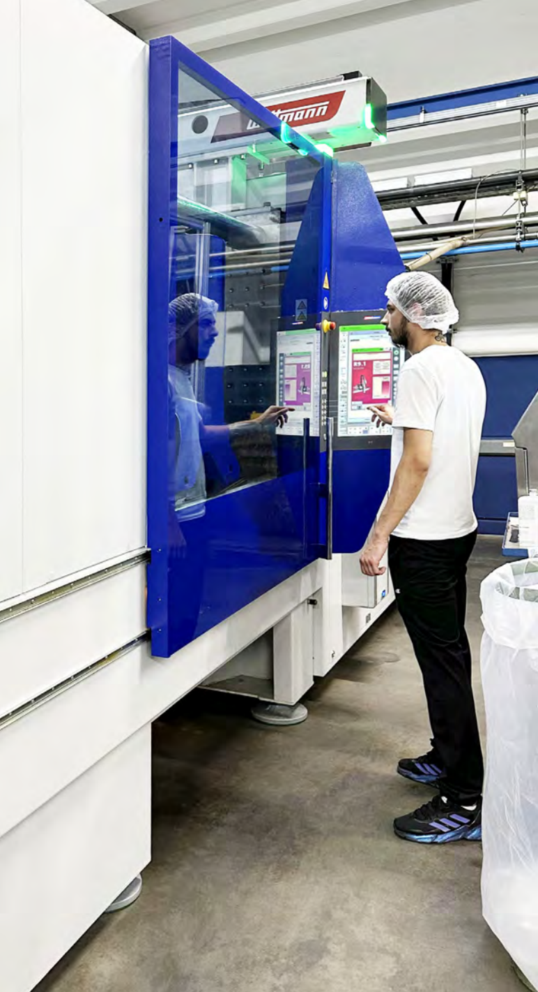
The control system integration of both the injection molding machine and the robot facilitates operation of the production cell.
