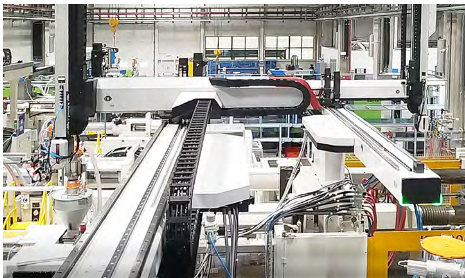
Two W843 pro robots remove two parts from two neighboring machines at different times.
