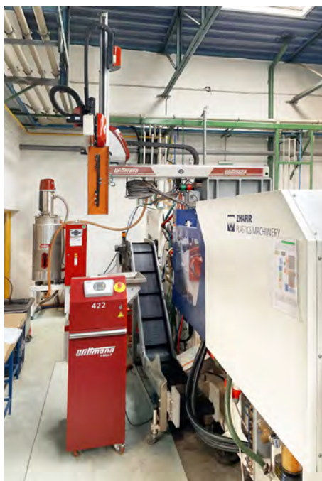
Central screenless granulator Junior Double 6 (top) and beside-the-press screenless granulator S-Max 2 in the SARTECH injection molding production area.
