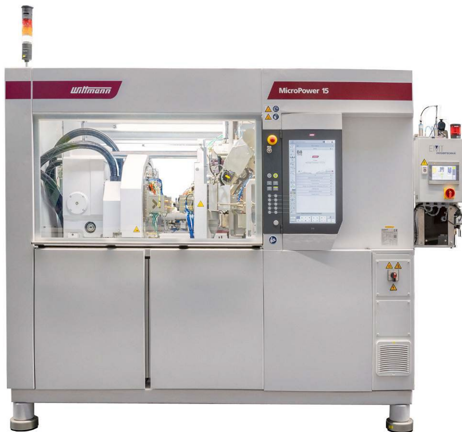
Fig. 1: MicroPower 15/10H/10H Combimould with LSR dosing pump
