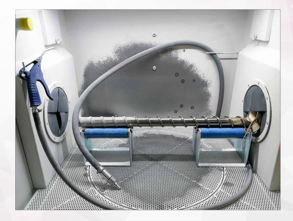
Our blasting system enables residue-free cleaning of components such as screws, nozzle heads, RSPs, nozzles, etc. that are heavily soiled with plastic.
