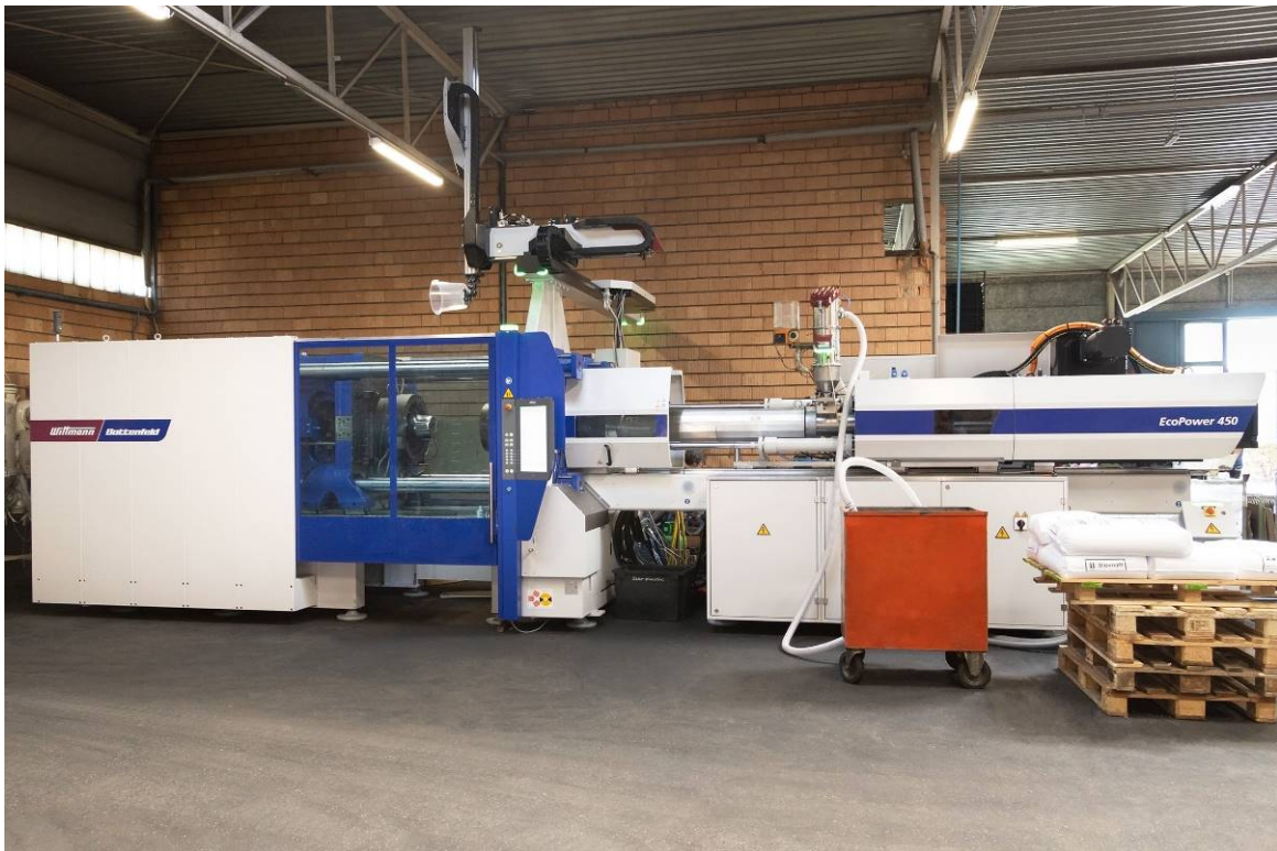
Fig. 1: EcoPower 450/3300 with WITTMANN FEEDMAX basic material loader and W832 pro robot just removing a finished bucket from the machine.
