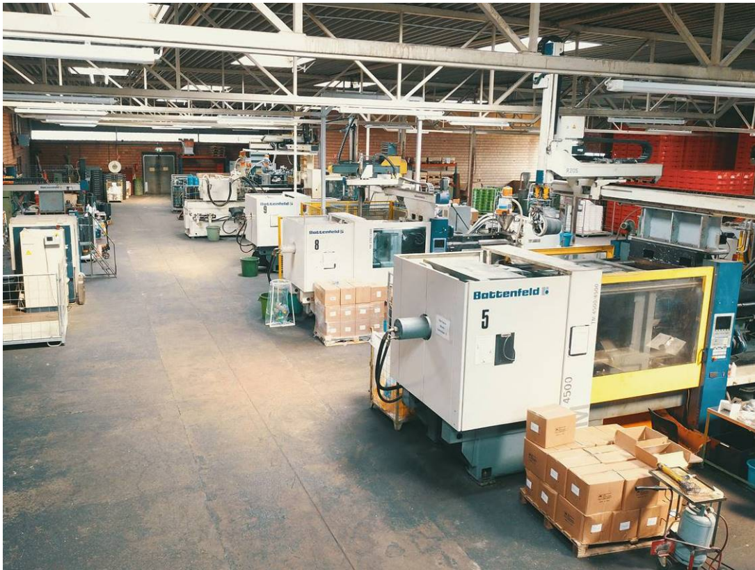
Fig. 2: Partial view of Teko-plastic's production floor located in Weiz/Preding. For the comparison of energy consumption with the EcoPower , a BATTENFELD TM 4500 injection molding machine was used (in the picture front right).
