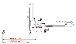
This diagram very clearly illustrates the difference between the reach and the X-stroke
