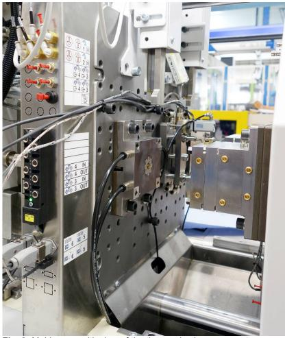
Fig. 3: Mold space with view of the thermoplastic component
