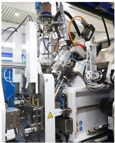
Fig. 2: 2-step screw-and-plunger aggregates of the MicroPower COMBIMOULD LIM
