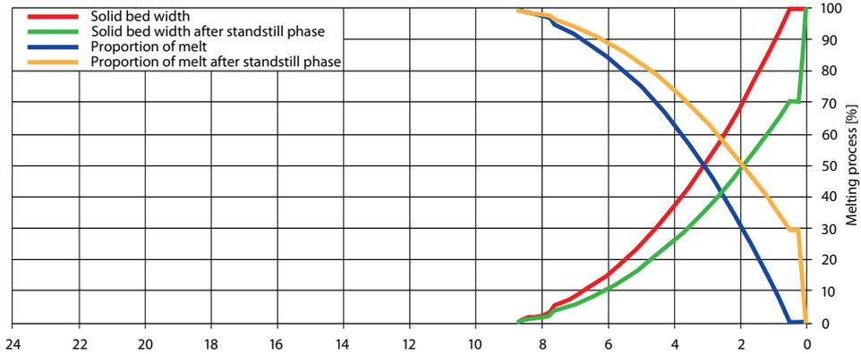
Melting process for the screw in stroke position 50 mm towards the end of the cycle: results of the original calculation prior to optimization.
