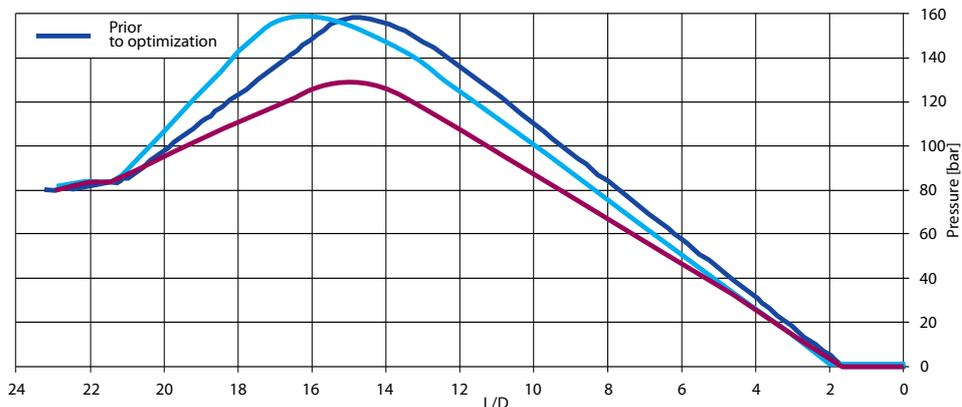
Pressure curves before and after the optimizations. Test 1: pressure curve at stroke position 50 mm. Test 2: increase of flight depth by approx. 28%.
