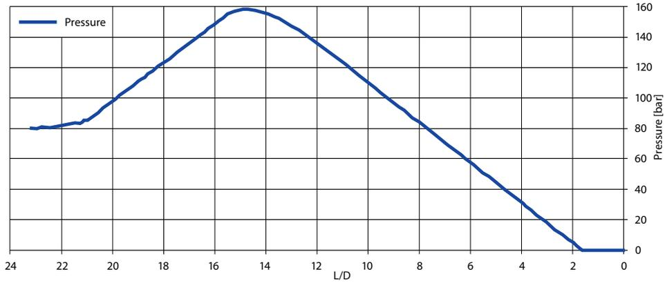
Pressure curve along the screw at 50 mm stroke position prior to optimization.
