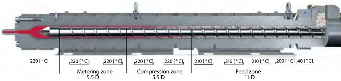
The calculations are based on the barrel zone temperatures.
