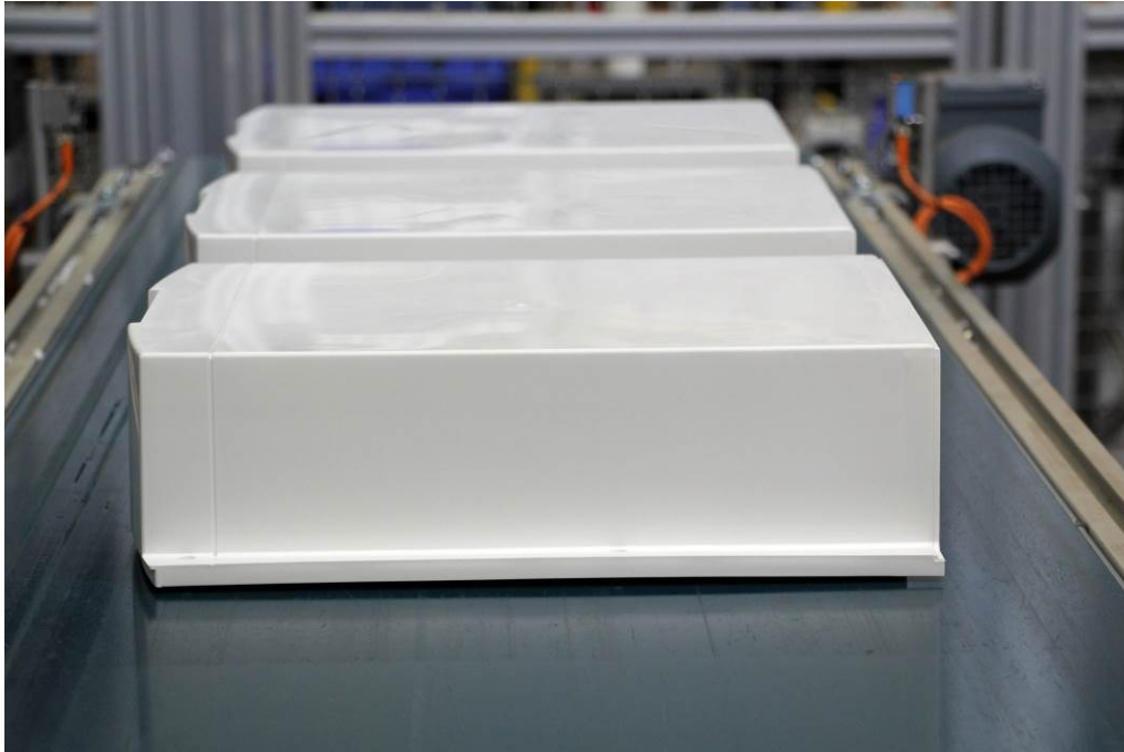
Fig. 4: Housing components for a wall storage heater – manufactured on the MacroPower 850
