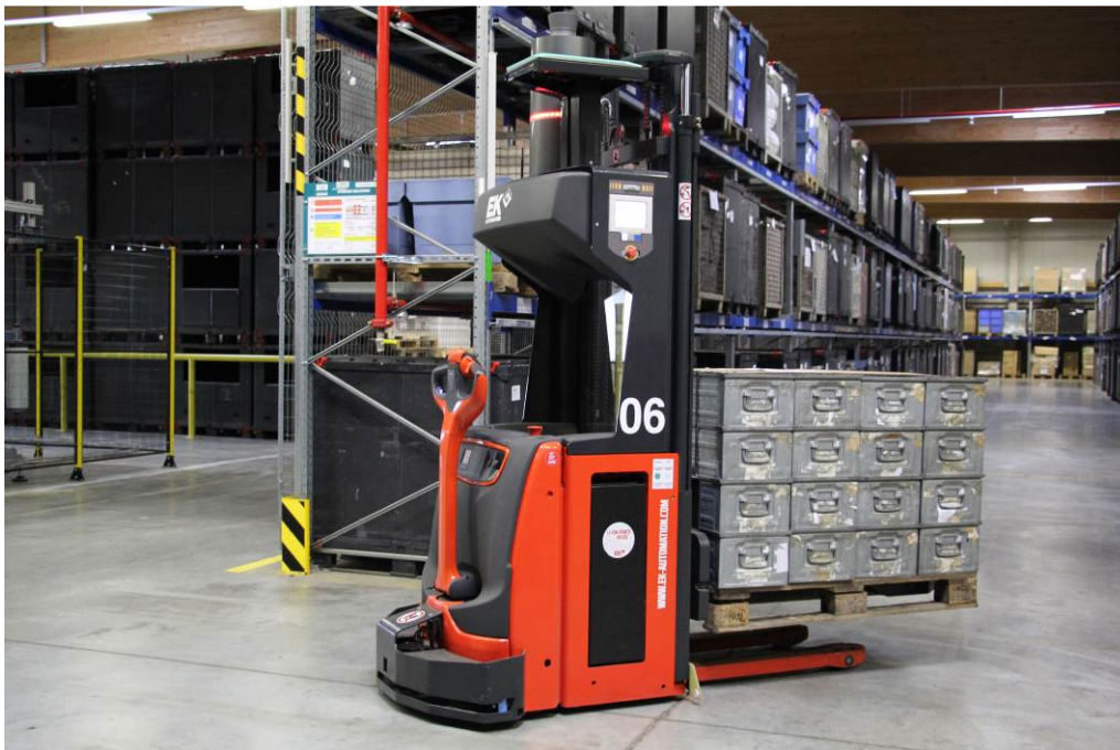
Fig. 3: Driverless transportation system at STIEBEL ELTRON
