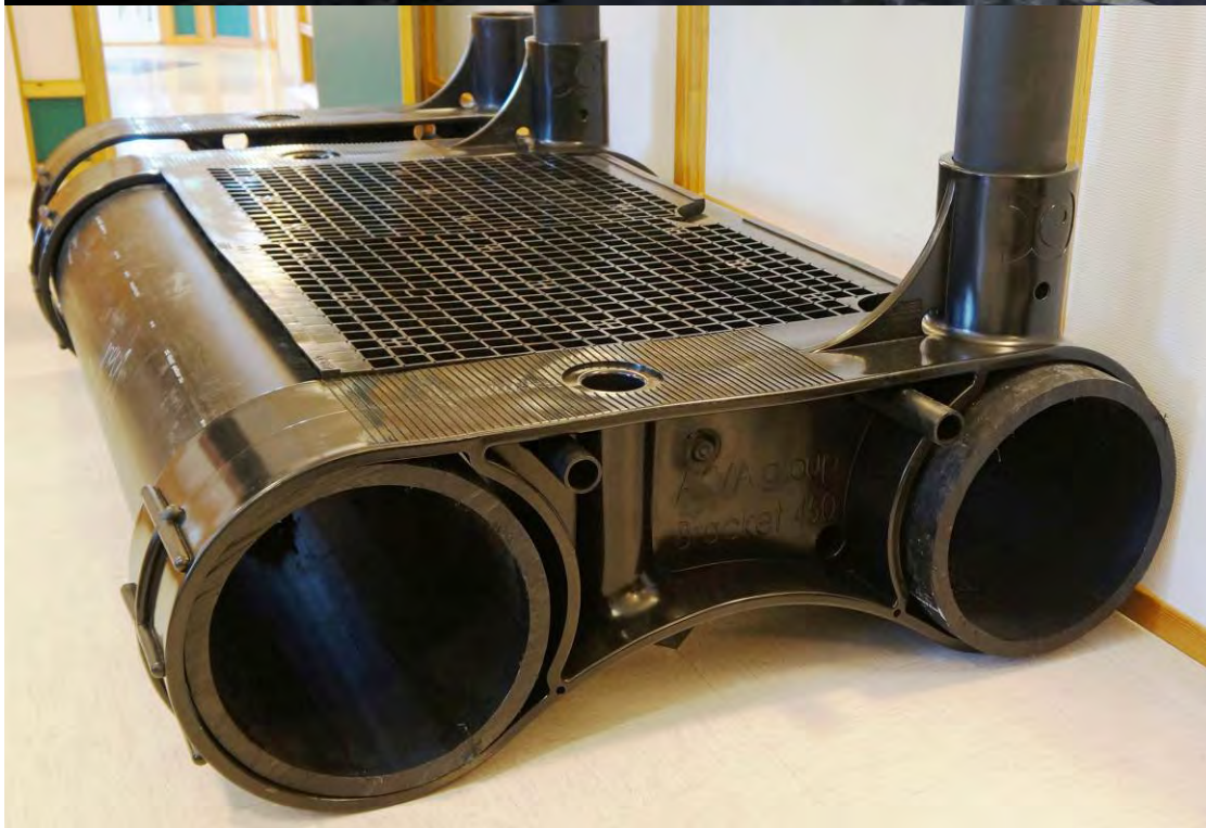
Fig. 2a+b: The core components of fish farms: two tightly welded plastic pipe rings as floats with diameters of 60 meters or more, which are held together and in position by brackets (2b).
