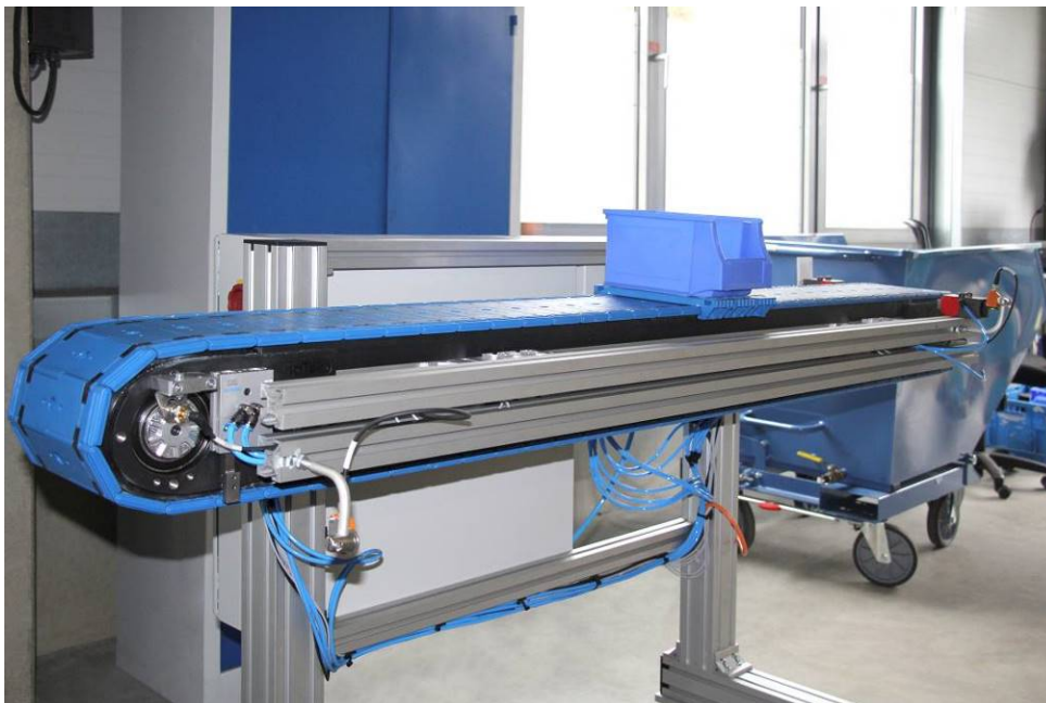
Fig. 5: Flexi conveyor (testing appliance) from ErgoTek consisting of plastic parts made by Happ (Photo: WITTMANN BATTENFELD)
