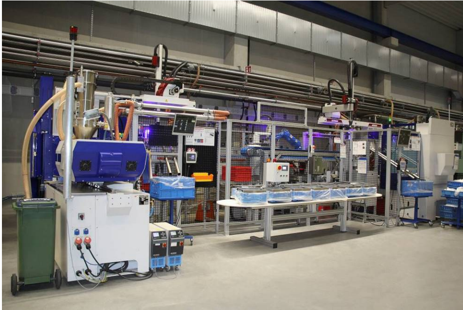
Fig. 2: General view of the EcoPower 110/350 injection molding machines from WITTMANN BATTENFELD linked together by conveyor systems with buffer capacity (Photo: WITTMANN BATTENFELD)
