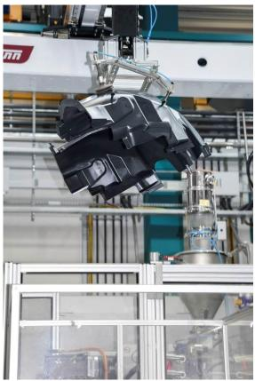
Fig. 4: Removal and depositing of a wheel arch liner by a WX173 robot from WITTMANN (Photo: WITTMANN BATTENFELD)
