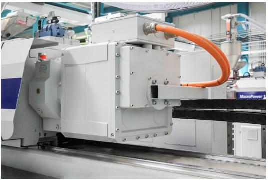
Fig. 3: Servo-electric screw drive on a MacroPower 2000 (Photo: WITTMANN BATTENFELD)
