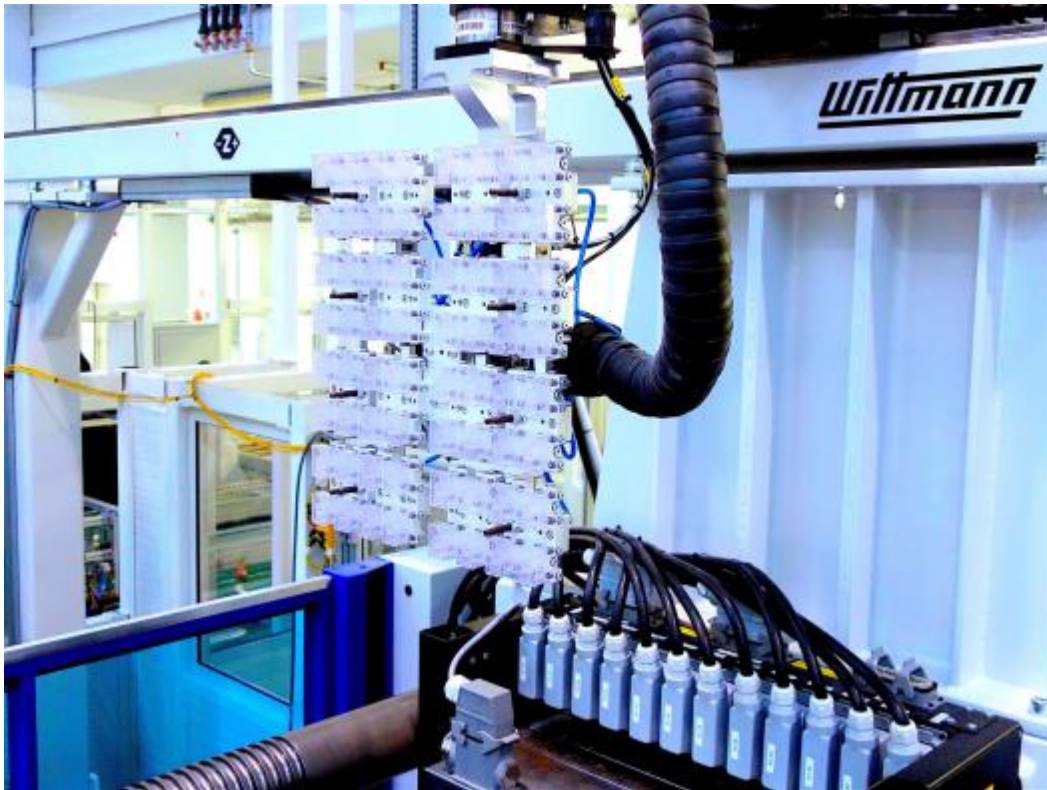
Fig. 5: 64-cavity hot-runner molds are used in production
