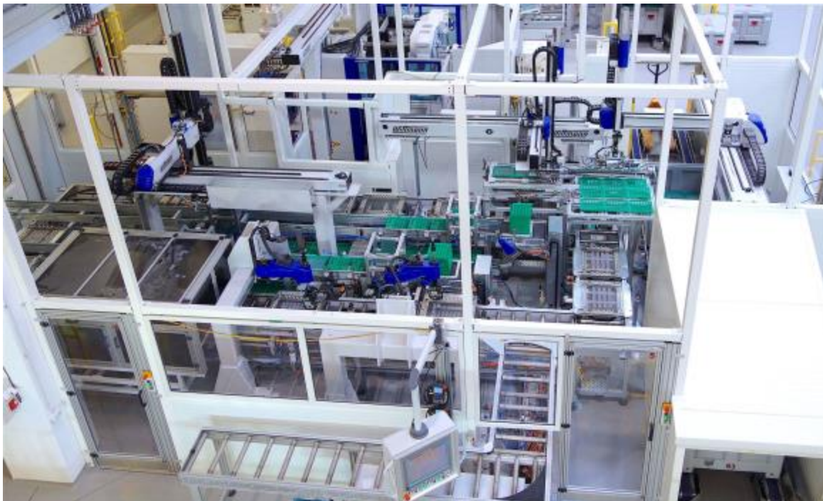
Fig.6: Every workpiece carrier passes through a vision control station (shown at the bottom on the left) for automatic scanning of every molded part from 5 directions
