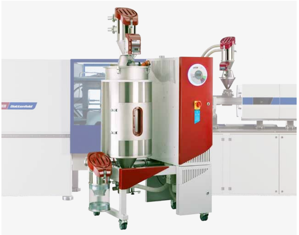
WITTMANN DRYMAX Aton BS/6 segment wheel dryer with draining function for the material pipeline to the machine, dry-air conveyance, demand- controlled material conveyance and adjustable input volume.
