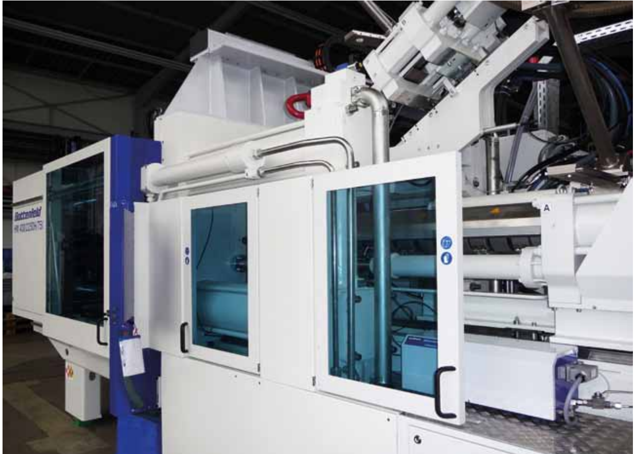
2-component CELLMOULD® injection molding machine with 400 metric tons of clamping force.
