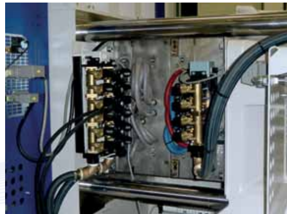
Correction of the mold temperature by addressing the individual cooling circuits of the WITTMANN FLOWCON flow controller.
