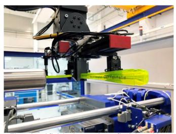
The printed finished part prior to final depositing.
