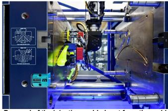
Removal of the injection-molded part from the mold.
