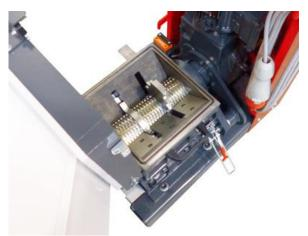
S-Max 2, opened: view of the cutting chamber.
