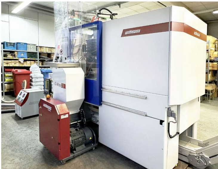
Fig. 6: Sprue is granulated directly. For making the drugstore items, up to 10% regrind can be blended in with the virgin material.
