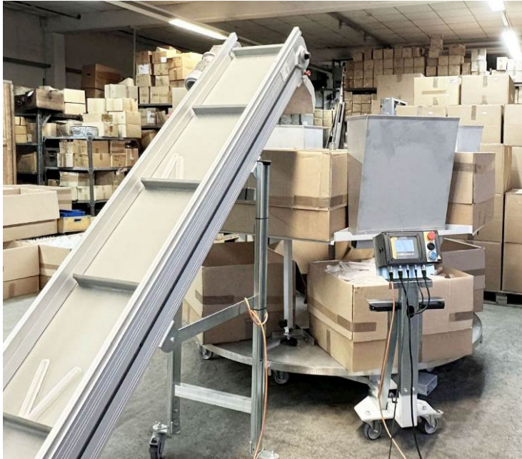
Fig. 5: The two-level product carousel makes autonomous production for up to 18 hours possible.
