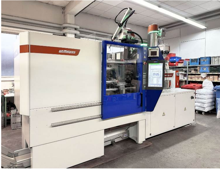
Fig. 3: The core of the production cell is a SmartPower injection molding machine with a sprue picker. Thanks to the high energy efficiency of the servo-hydraulic machine, RING Kamm und Haarschmuck was able to benefit from the German government's public funding program.
