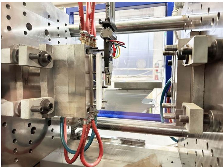
Fig. 4: The comparatively large mold platens of the SmartPower injection molding machine offer ample flexibility for mounting a great variety of molds including relatively large specimens.
