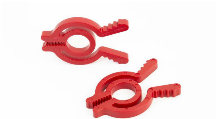
Fig. 2: With Airmould internal gas pressure technology, the production of clothes pegs made of polypropylene requires 26.3 per cent less raw material compared to compact injection molding. The weight of the finished parts is reduced by the same percentage.
