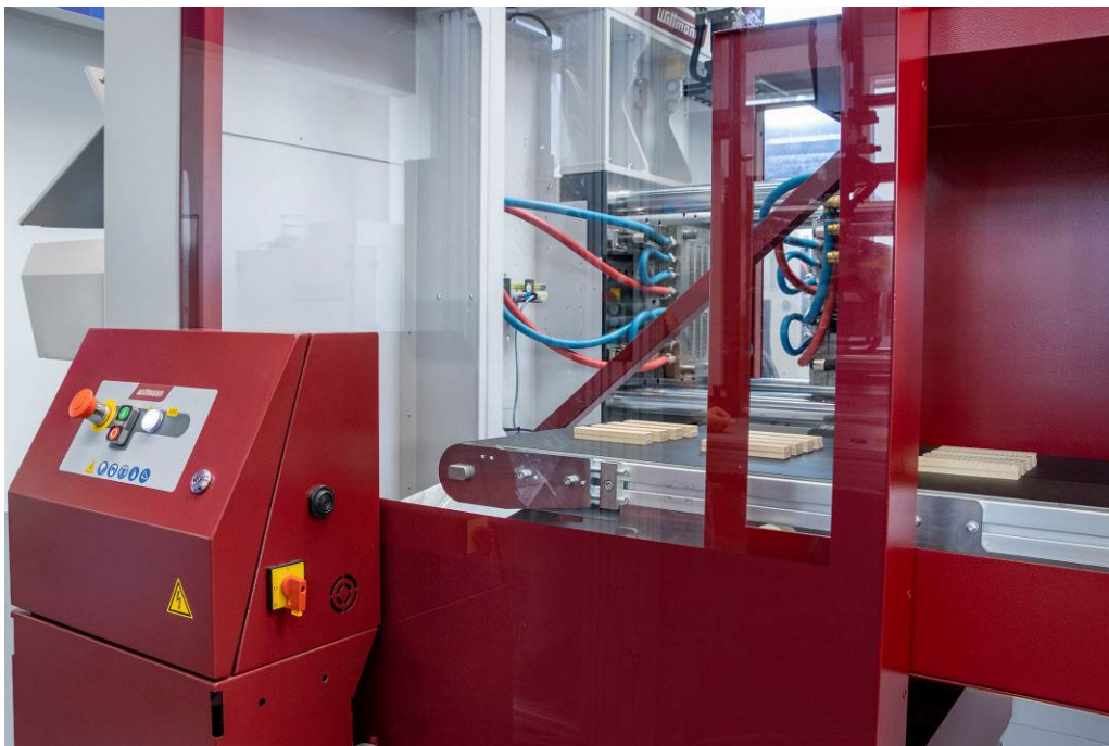
Fig. 3: EcoPower 110/350 B8X equipped as an Insider cell with an S-Max 3 screenless granulator
