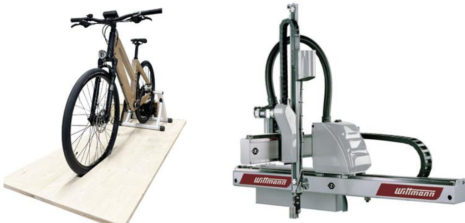
The adapted bike of the ErgoRobot application and the Primus 14 robot from WITTMANN driven by it.
