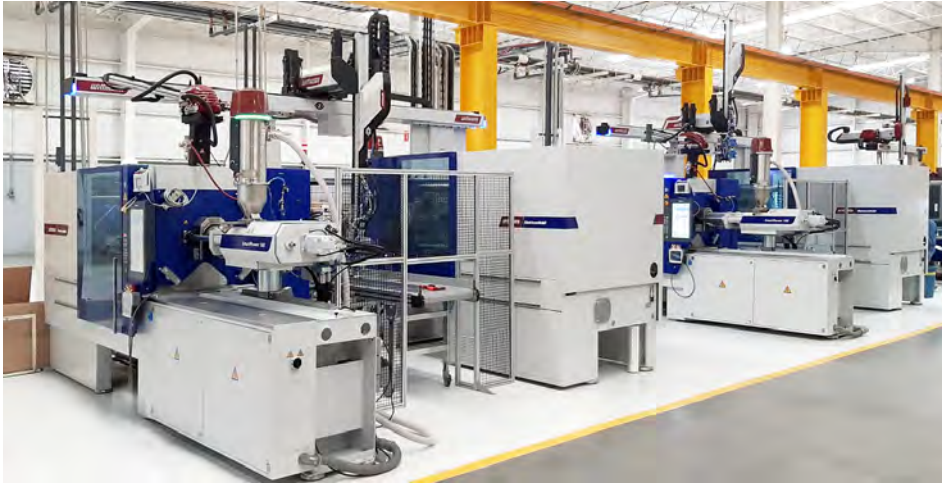
View of an ISGO production hall, housing the WITTMANN two-machine working cell for the production of shell type handles for a screw driller.
