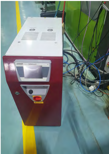
After: A Tempro plus D L120 temperature controller (the "L" in the name stands for "large") with a frequency-controlled 4.0 kW pump with a max. capacity of 300 l/min, a max. heating performance of 36 kW, as well as a direct cooling capacity of up to 250 kW. Here, the medium water is distributed to 16 cooling circuits via a 2 x 8-fold WFC 100 (WFC = Water Flow Control).
