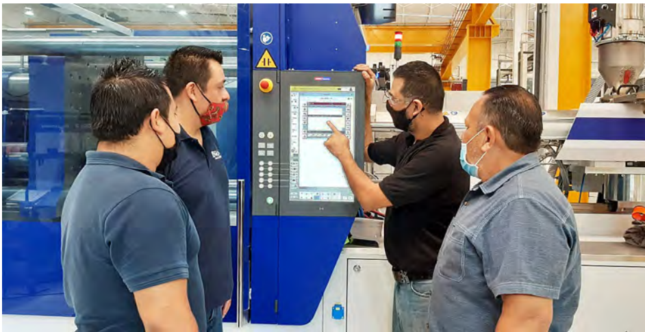
ISGO operators, working on the Unilog B8 control of a SmartPower injection molding machine.
