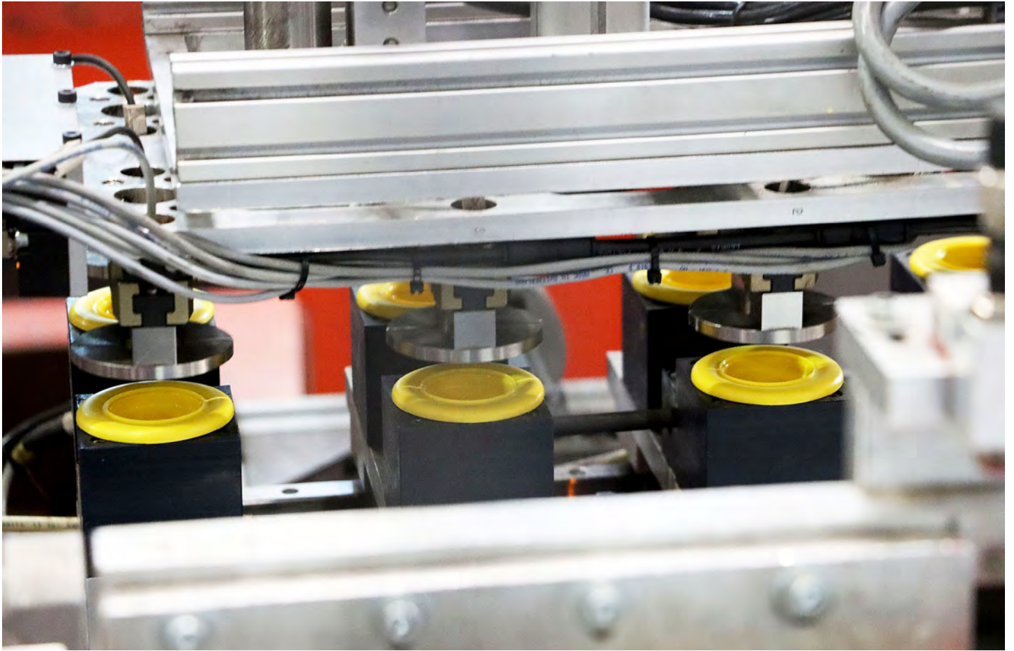
The gripper of a WITTMANN robot picking up the wheel rims of toy cars.
