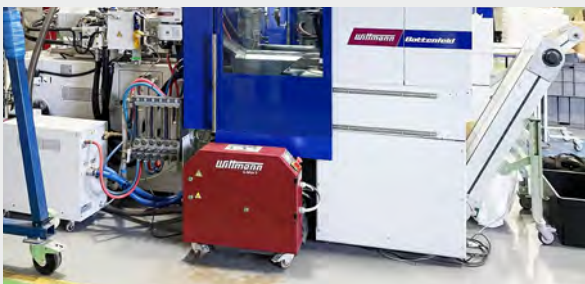
Page 4: Ingrinder solution for space-saving recycling by Rugby Plastics in Leicester, UK.
