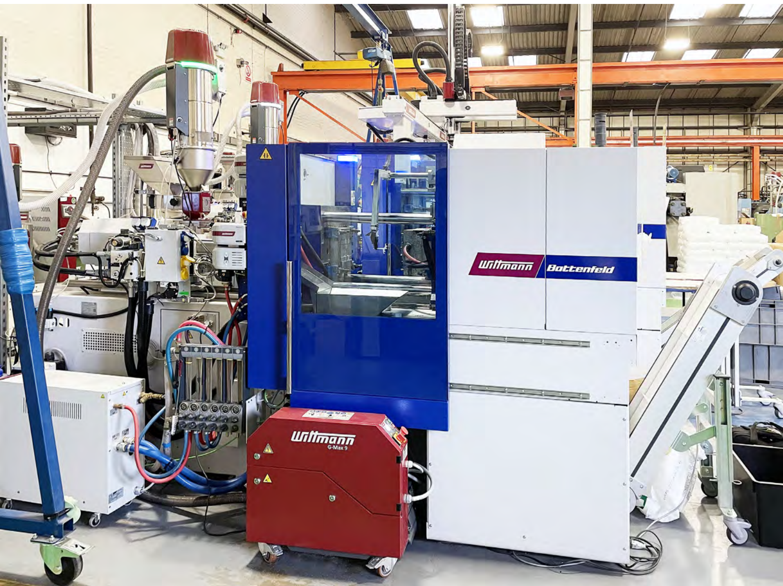
SmartPower 60 Ingrinder system, consisting of a SmartPower injection molding machine with 60 tons of clamping force, a G-Max 9 granulator, a Feedmax S3 net material loader, a TEMPRO temperature controller, and a sprue gripper from the WITTMANN Group – installed at the Rugby Plastics plant in Leicester, UK.
