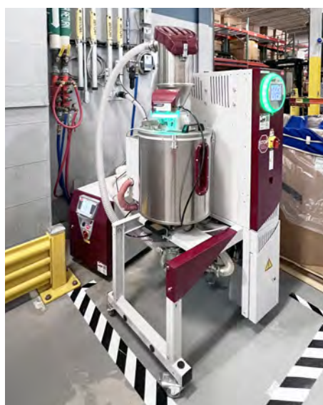
WITTMANN dry air dryer with FEEDMAX material loader, and with TEMPRO temperature controller behind it.
