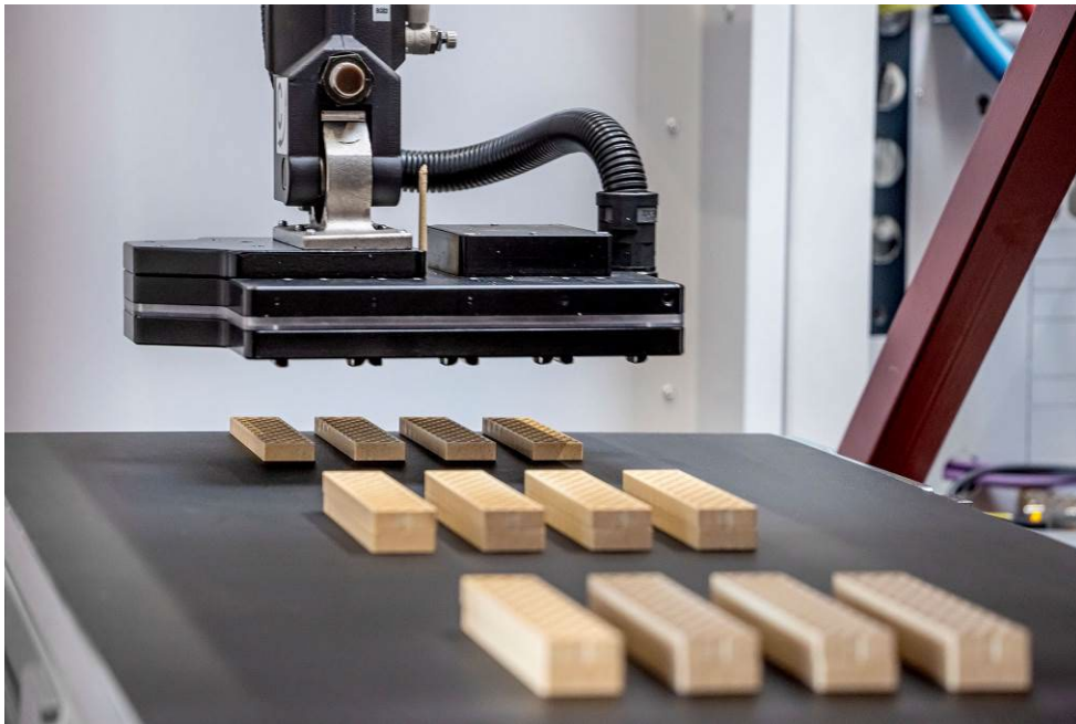
Fig. 3: The parts are stacked and deposited on a conveyor belt.
