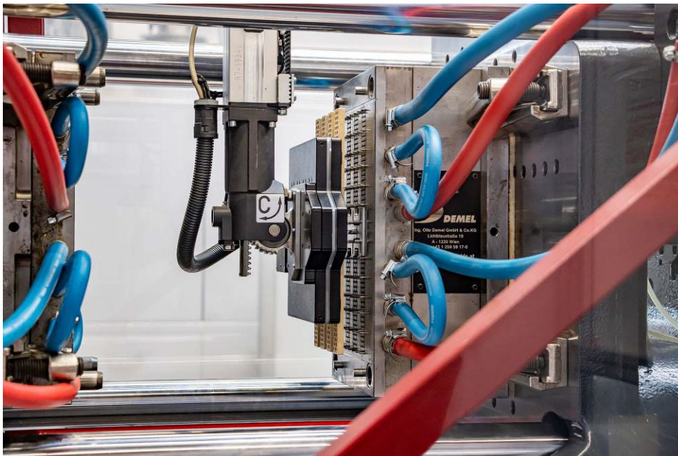
Fig. 2: Removal of parts with WITTMANN robot W918
