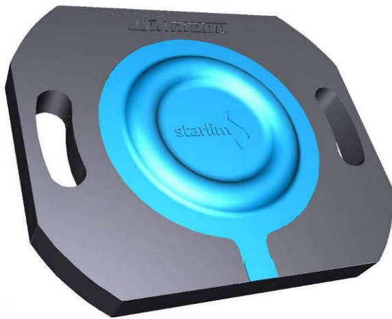
Figs. 7a+b: Membrane made of thermoplastic and liquid silicone for a high-quality micro loudspeaker, manufactured on a MicroPower 15/10H/10H Combimould (photos: Starlim Spritzguss GmbH)
