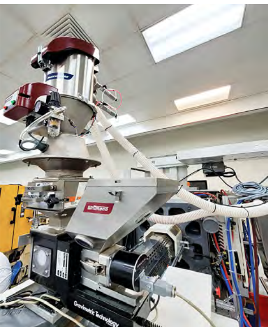
FEEDMAX loaders conveying resin that is dried outside of the clean room.
