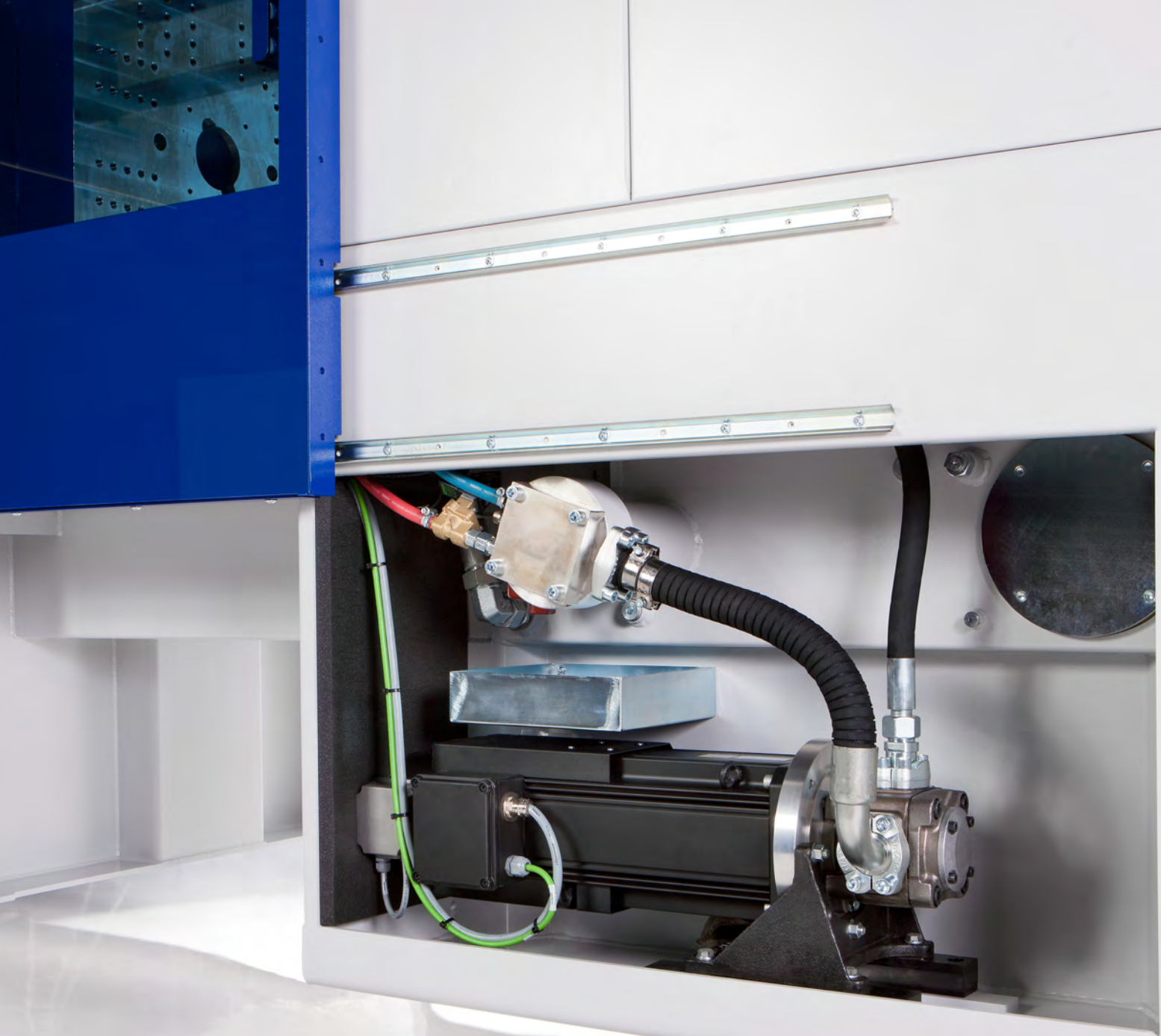
View of the servo drive (right half of the picture) of a WITTMANN BATTENFELD SmartPower injection molding machine.
