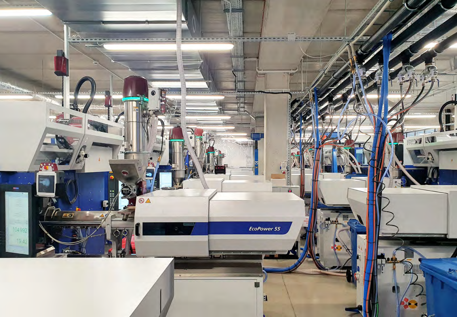
Views of the new NOEX production hall in Komorniki, Poland for COVID test kits, with 16 EcoPower 55/350 Insider injection molding machines from WITTMANN BATTENFELD.
