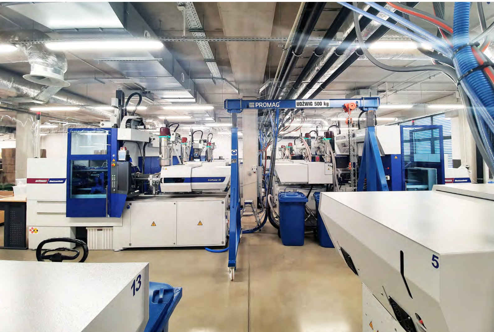
Views of the new NOEX production hall in Komorniki, Poland for COVID test kits, with 16 EcoPower 55/350 Insider injection molding machines from WITTMANN BATTENFELD.
