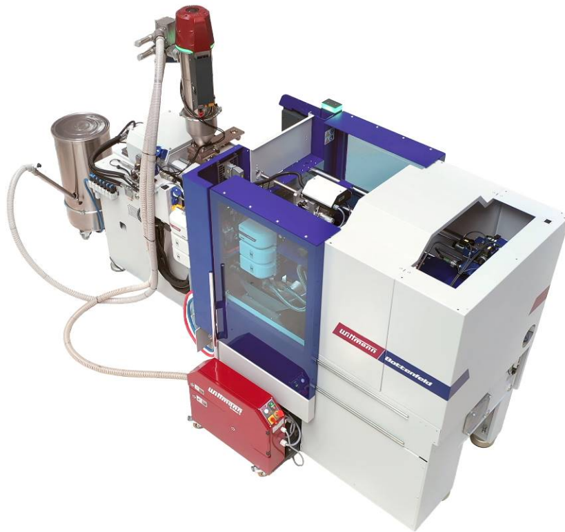
Fig. 3: Ingrinder with integrated G-Max 9 granulator
