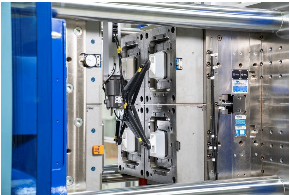
Fig. 2: EcoPower Xpress 300/1100+ – demolding of margarine tub
