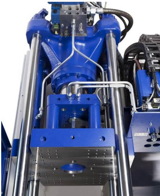
Fig. 2: Central hydraulic clamping system of the SmartPower
