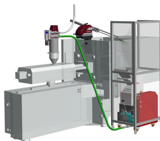
Drawing of an inline recycling cell with sprue picker, granulator and material loader
