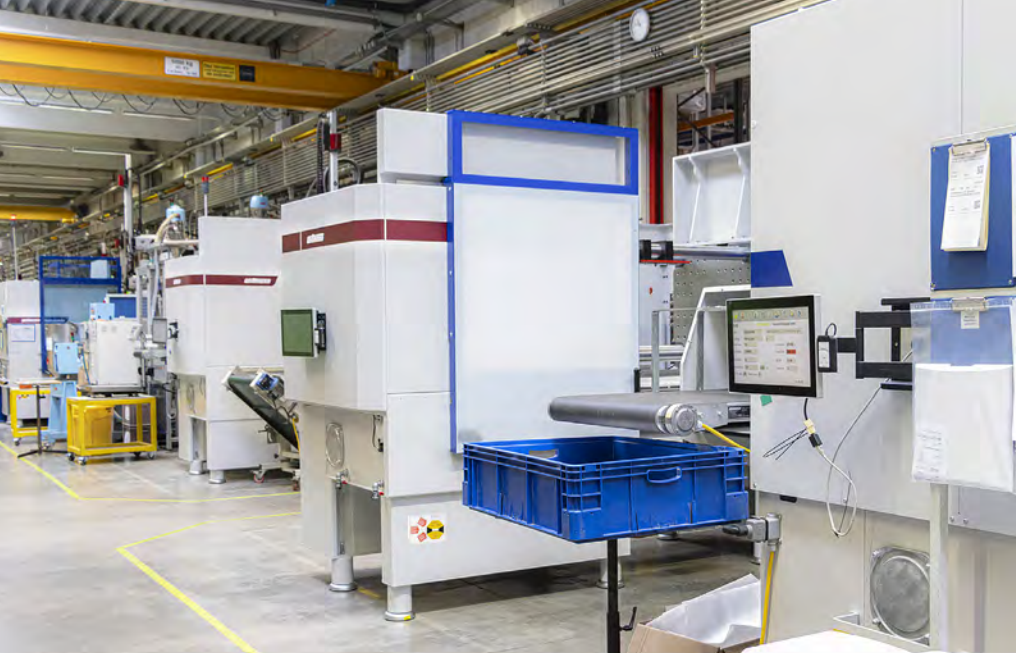
View of the FUSO Production in Ybbsitz, Lower Austria: SmartPower machines from WITTMANN BATTENFELD designed as Insider cells with WITTMANN linear robots.
