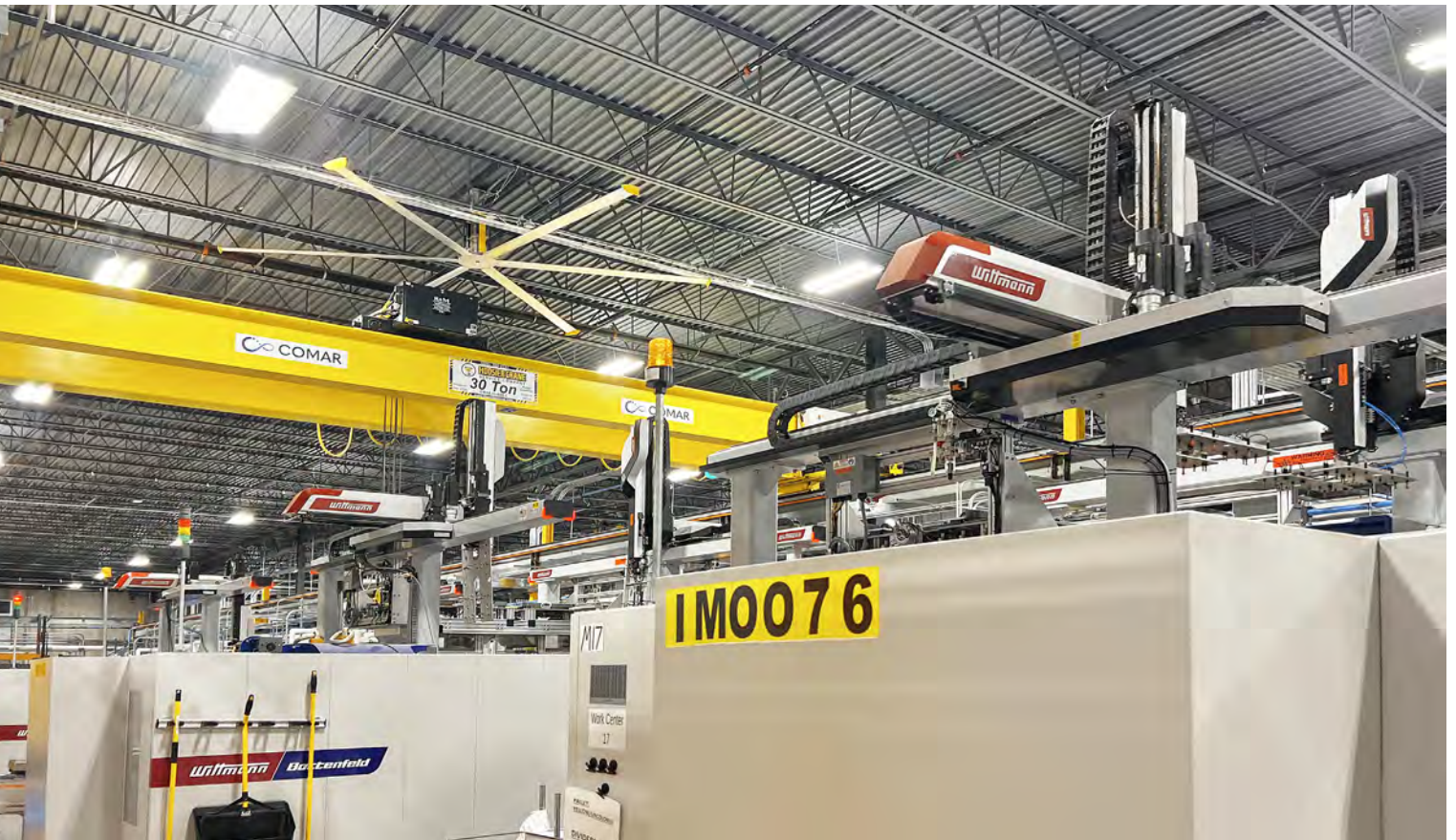
Each of the four new machines at Comar in West Bend is equipped with two W833 pro high-speed robots.
