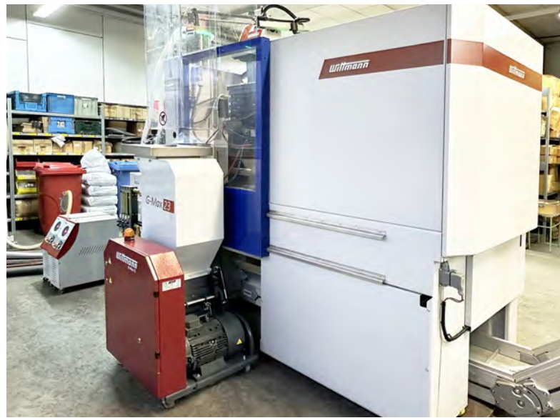
Picture left: The two-level product carousel makes autonomous production for up to 18 hours possible. Picture right: Sprue is granulated directly. For making the drugstore items, up to 10% regrind can be blended in with the virgin material.
