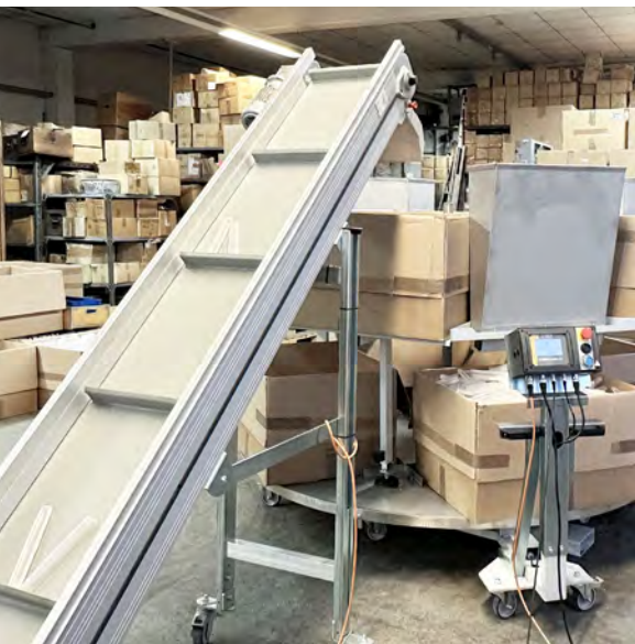
Picture left: The two-level product carousel makes autonomous production for up to 18 hours possible. Picture right: Sprue is granulated directly. For making the drugstore items, up to 10% regrind can be blended in with the virgin material.
