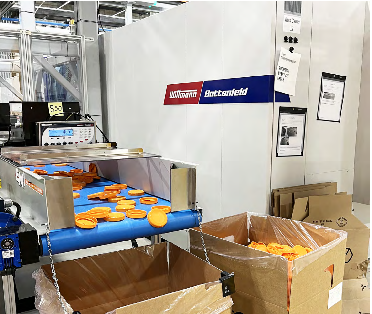
Thin-wall lids for round containers are produced on WITTMANN Group injection molding machines at Comar's West Bend, Wisconsin plant.
