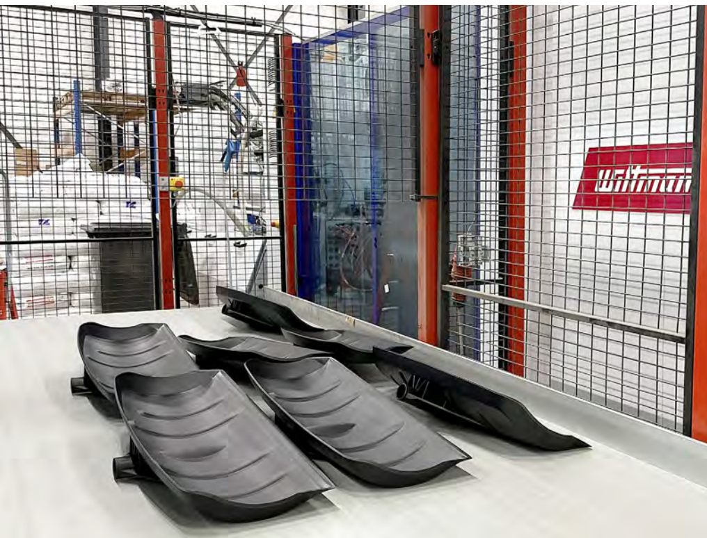
The blades of the feeding shovels are manufactured on a MacroPower 850.
