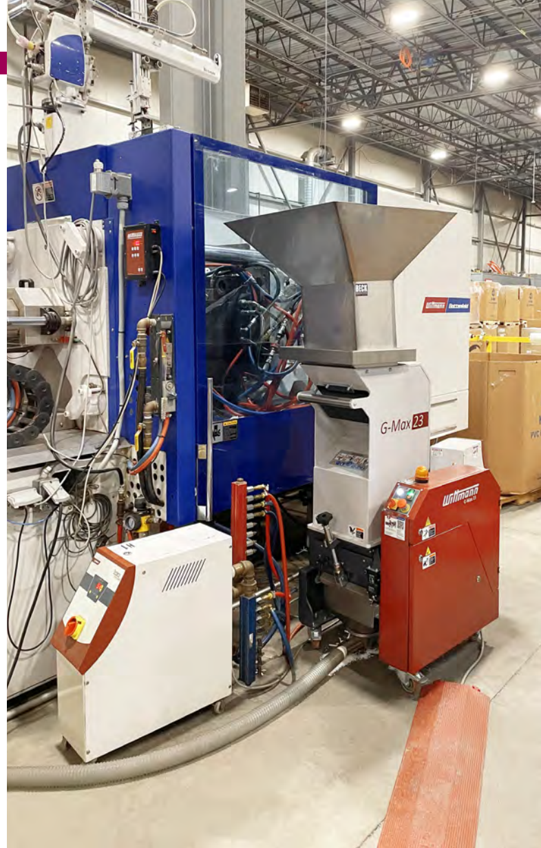
TEMPRO primus C120 temperature controller and G-Max 23 granulator, next to an EcoPower 240 molding machine.
