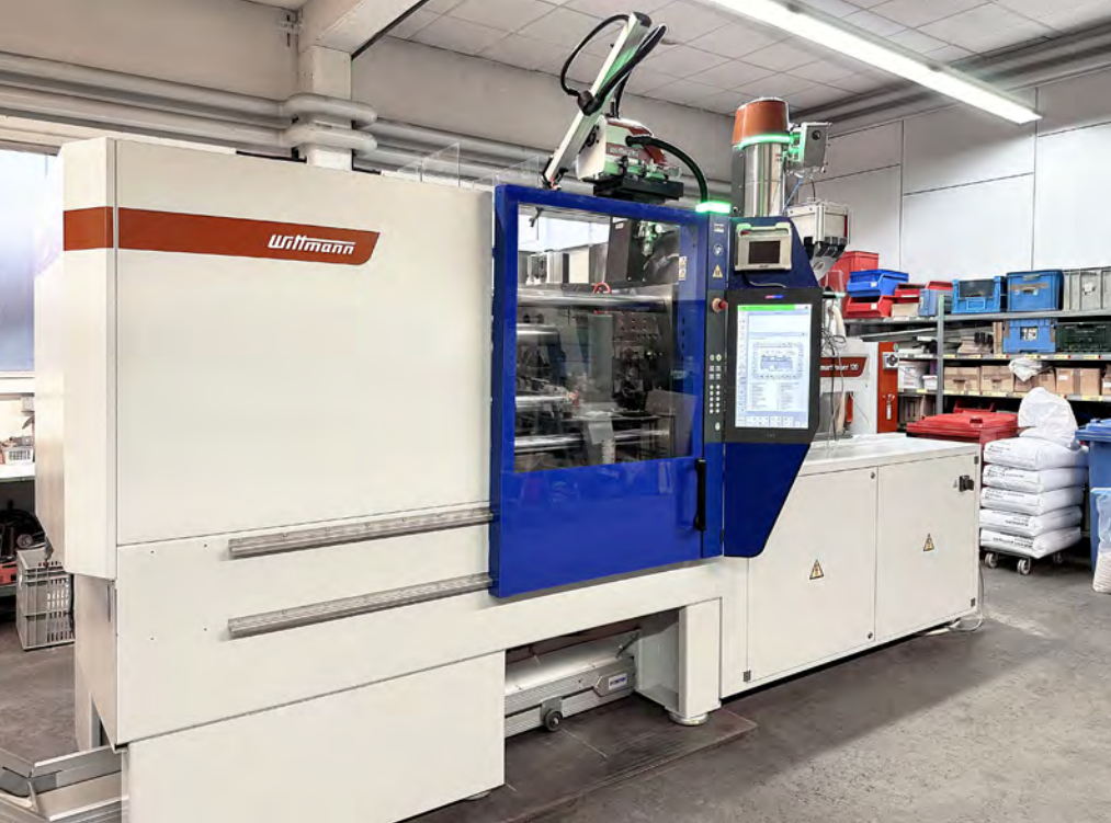
The core of the production cell is a SmartPower injection molding machine with a sprue picker. Thanks to the high energy efficiency of the servo-hydraulic machine, RING Kamm und Haarschmuck was able to benefit from the German government's public funding program.
