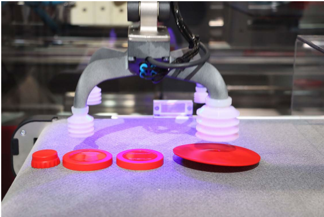
Fig. 3: LSR covers for beverage containers
