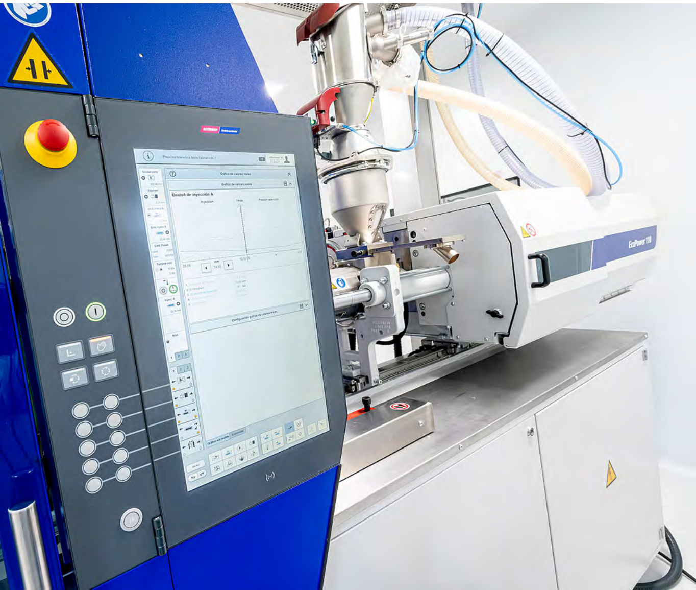
Unilog B8 control on EcoPower 110 injection molding machine. The Unilog B8 control system works with the Windows™ 10 IoT operating system, which provides extensive process control capabilities.
