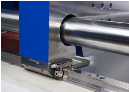
The cover shows the linear guide of a WITTMANN BATTENFELD injection molding machine.
