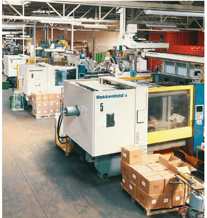
Partial view of Teko-plastic's production floor. For the comparison of energy consumption with the EcoPower, a BATTENFELD TM 4500 was used (in the picture front right). (Photo: Teko-plastic)
