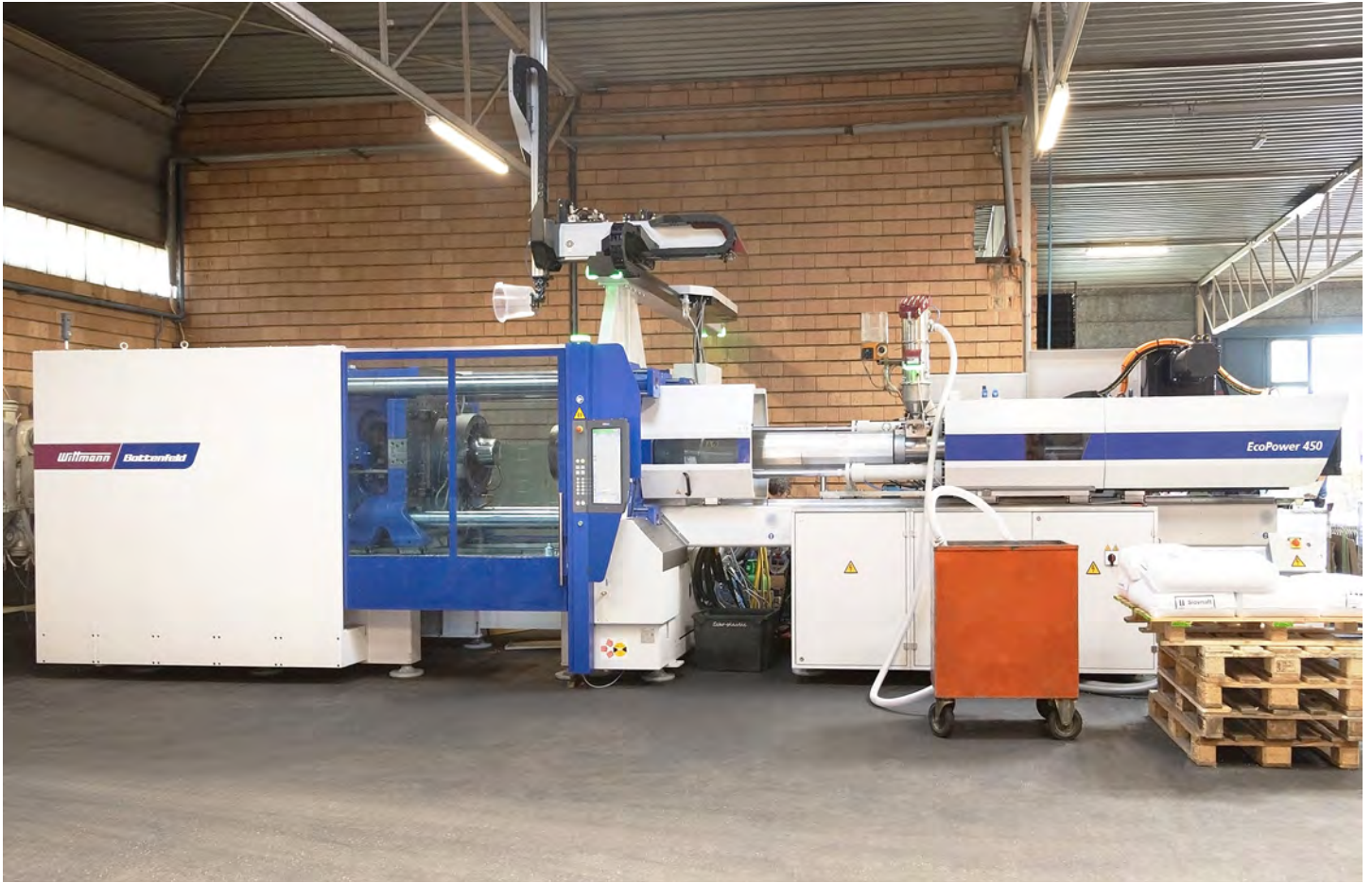
EcoPower 450/3300 with WITTMANN Feedmax basic material loader and W832 pro robot just removing a finished bucket from the machine. This bucket with a volume of 10 liters is produced on both machines for the purpose of comparison.
