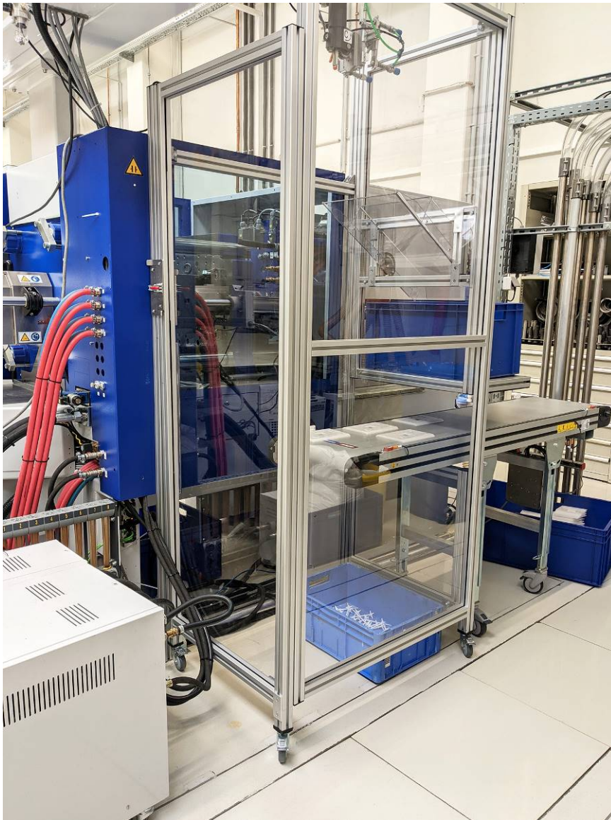
Fig. 1: Injection molding machine with Easy Cell
