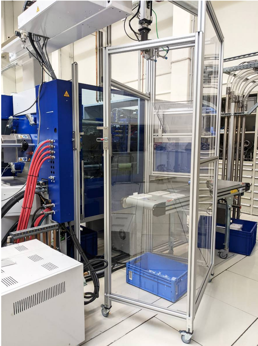
Fig. 2: Easy Cell shifted to provide access to the mold
