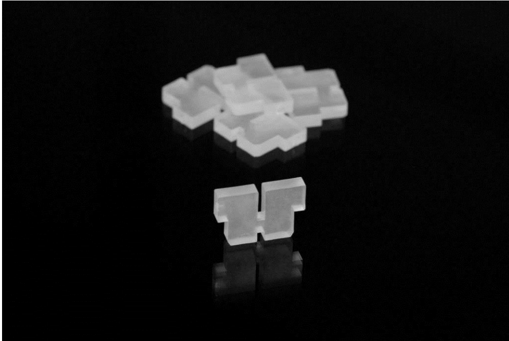
Fig. 5: High-precision Teflon parts to be built into high-frequency components
