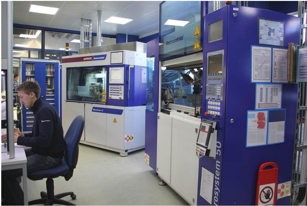
Fig. 1: High-precision micro injection molding at Rohde & Schwarz in an air-conditioned room
