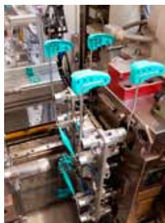
4 When the mold opens, the gripper removes the two finished parts with molded holders from the moving mold half (left), and loads the two other parts without holders into the fixed half (right).
