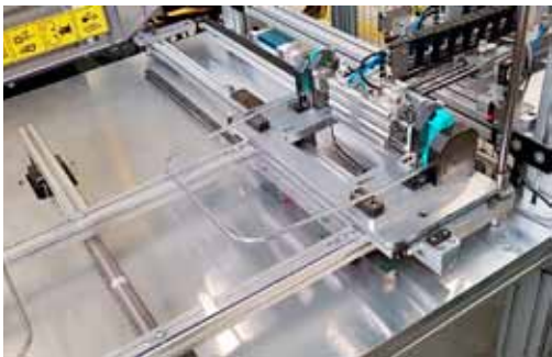
2 After loading, the station puts together the arched handles and the hinges by pressing.
