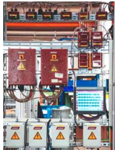
Picture left: Close-up view of the RFID-coded coupling station. Picture right: The system's "brain": bus modules, line server, and the WITTMANN touch-screen network control.
