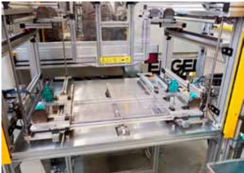
1 The production of the components is done in a double injection mold. First, the operator loads two metal arched handles into the insert preparation station, each with two mounted plastic hinges.
