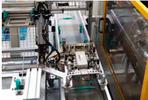
5 The gripper takes out the finished parts and one sprue from the mold area. The three parts are placed on a conveyor belt between the back side of the machine and the insert preparation station.
