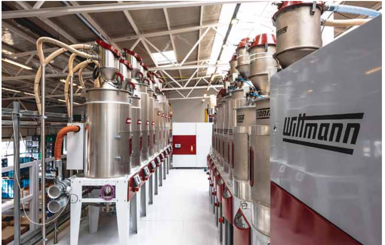
WITTMANN battery dryer and SILMAX drying hoppers with FEEDMAX material loaders, mounted on a platform in the WAREMA PT production plant in Gyál, Hungary.
