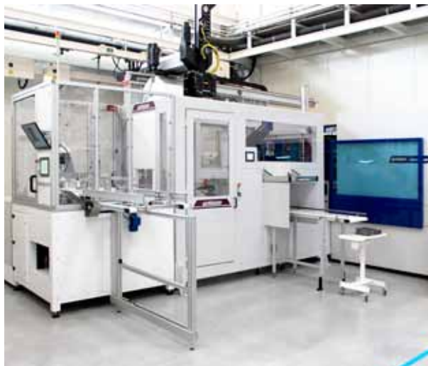
Complete workcell installation at Stiplastics Healthcaring in Saint-Marcellin, France: WITTMANN BATTENFELD SmartPower injection molding machine with 300 t of clamping force, WITTMANN W832 pro robot, and IML system.
