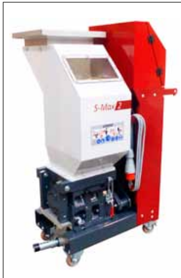
Picture left: Low-speed screen- less granulator S-Max 2, one of the three new models of the S-Max series. Picture right: FLOWCON plus stand-alone flow control solution from WITTMANN.
