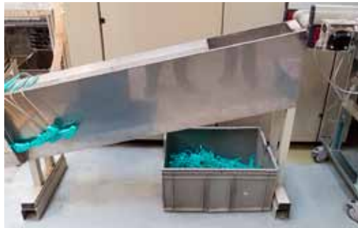
6 From the belt conveyor, the components slip down a special chute, driven by their own weight. The operator collects the parts from the chute.
