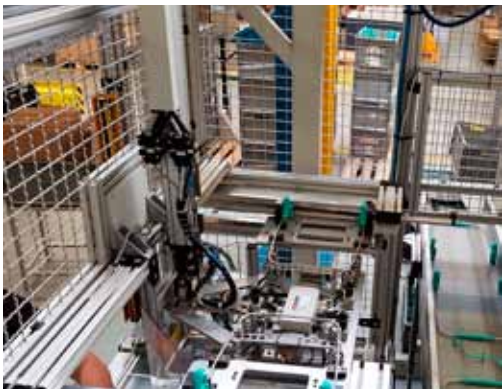
3 After having connected the parts to each other, the components are lifted, and taken by the insertion mechanism of the robot's gripper.
