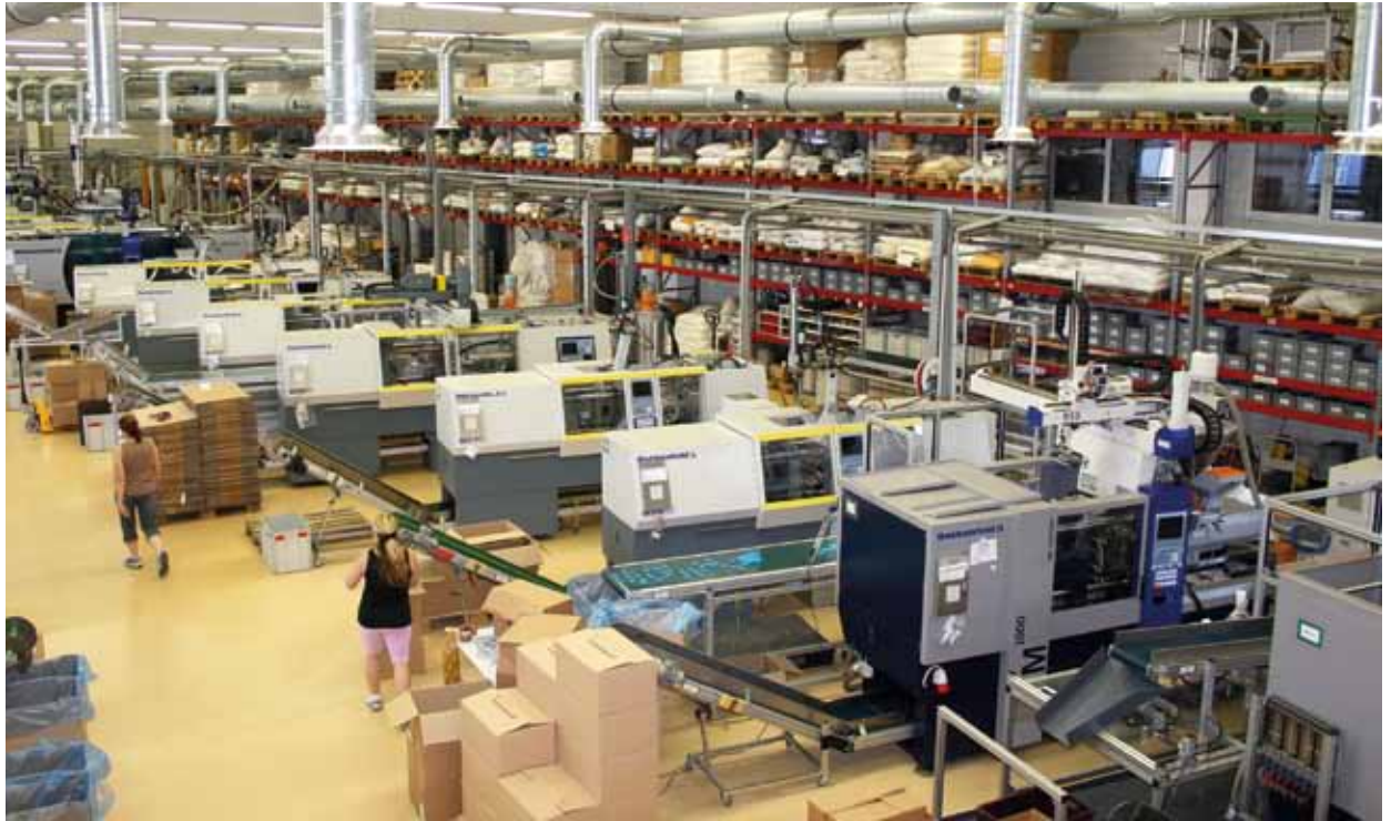
The LECHNER production hall no. 1 with 23 injection molding machines from WITTMANN BATTENFELD.
