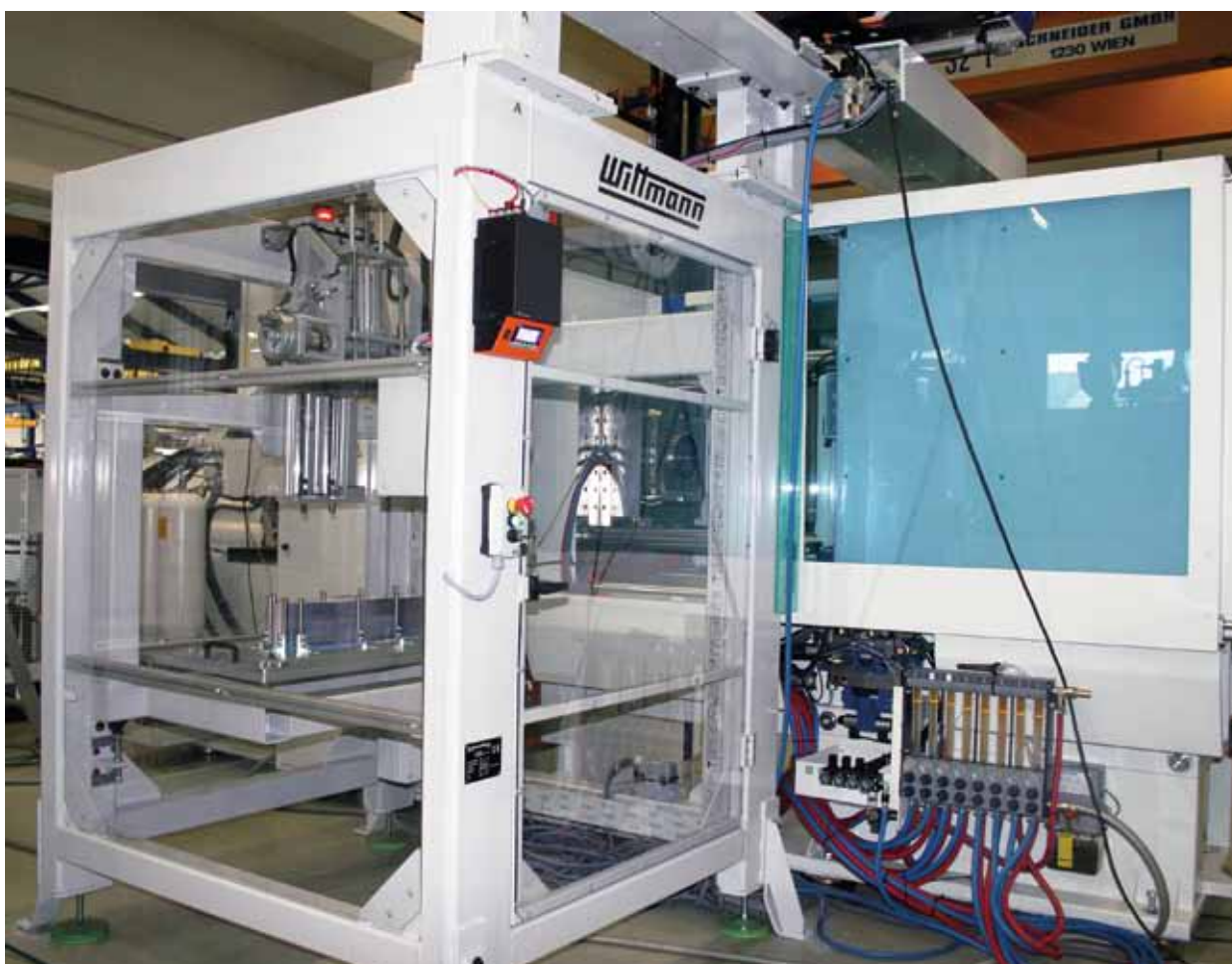
This view of one of the complete production cells at Tea Plast shows the TM injection molding machine from WITTMANN BATTENFELD and the WITTMANN W832 IML robot.
