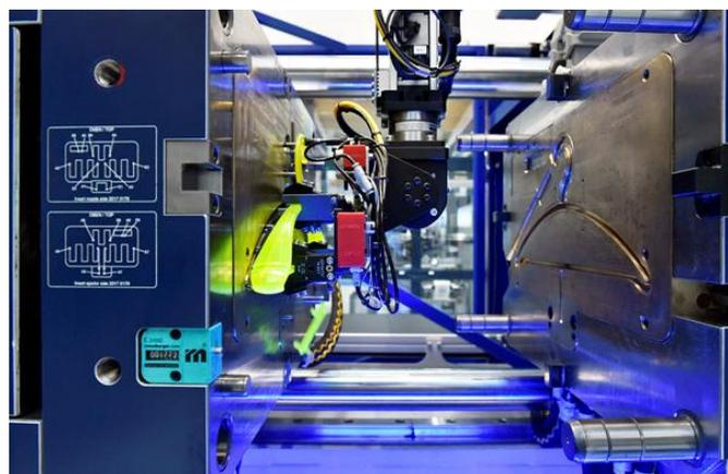
**Removal of the injection-molded part from the mold.**
