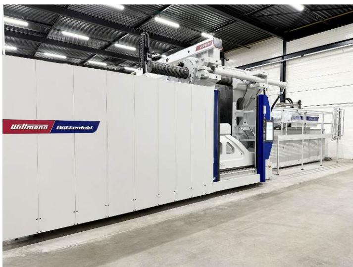
Fig. 6: The new MacroPower 2000 is the largest injection molding machine so far in AKROH's equipment. It is intended primarily for generating further growth in the business segment of contract injection molding.
