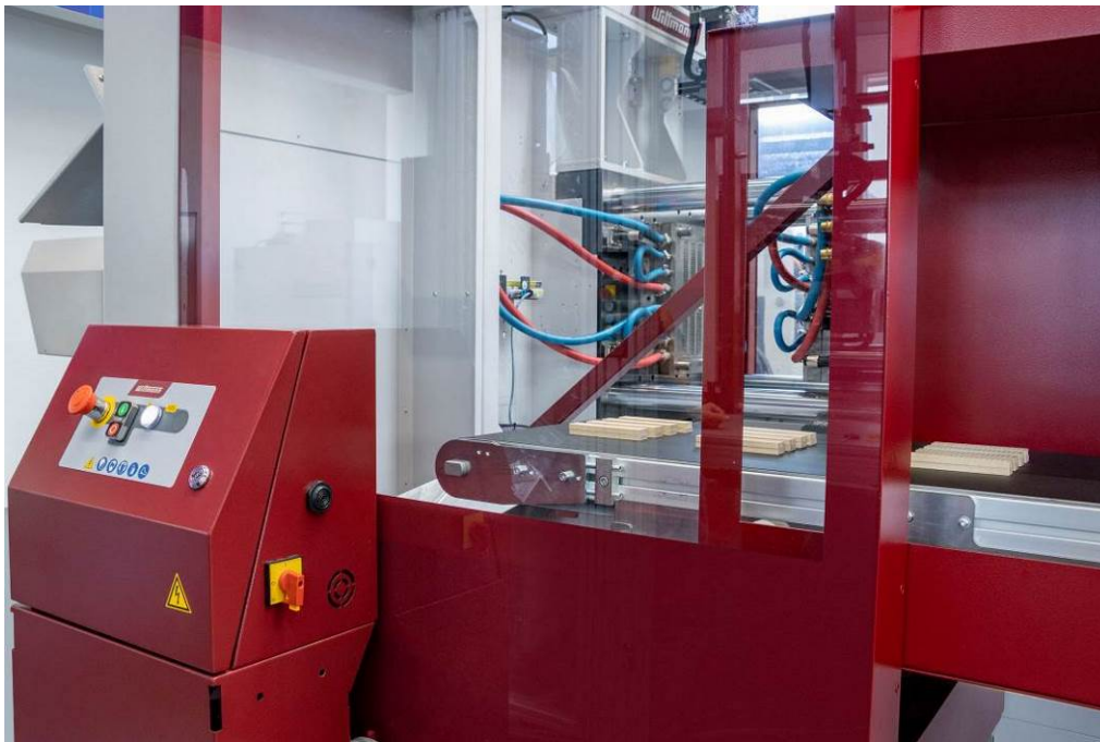
Fig. 1: EcoPower 110/350 B8X designed as an Insider cell with an S-Max 3 screenless granulator
