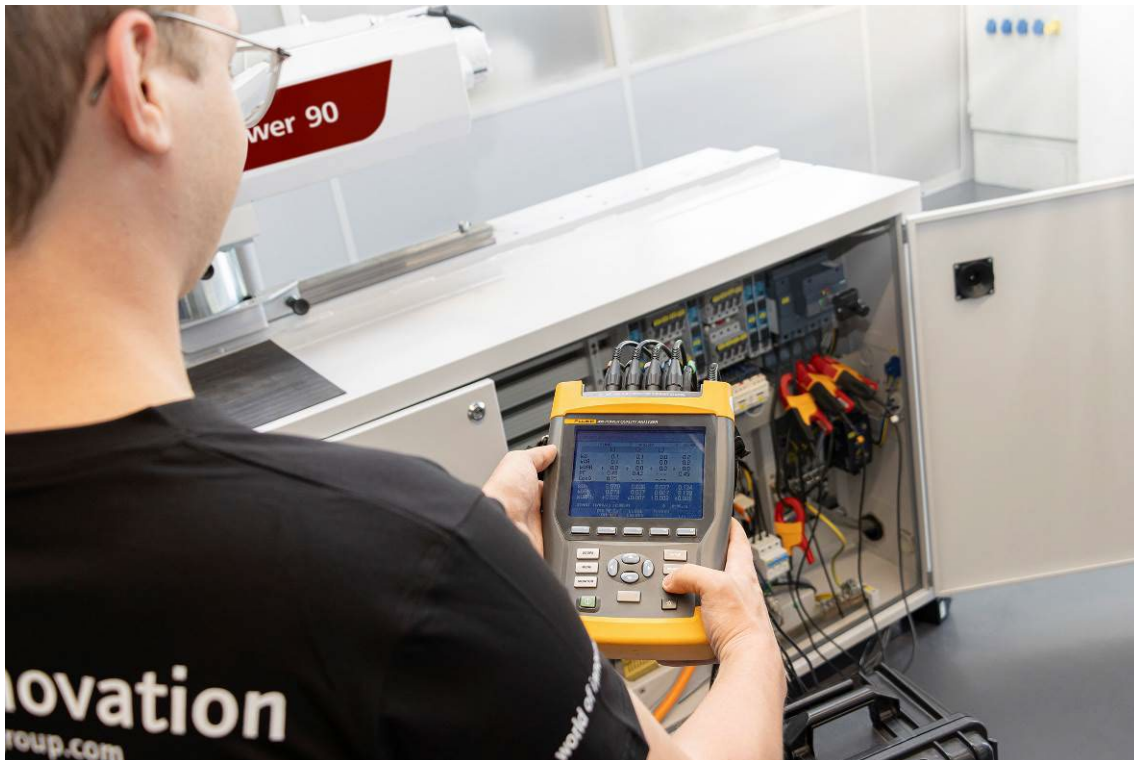
Fig. 3: Energy measurement on the machine
