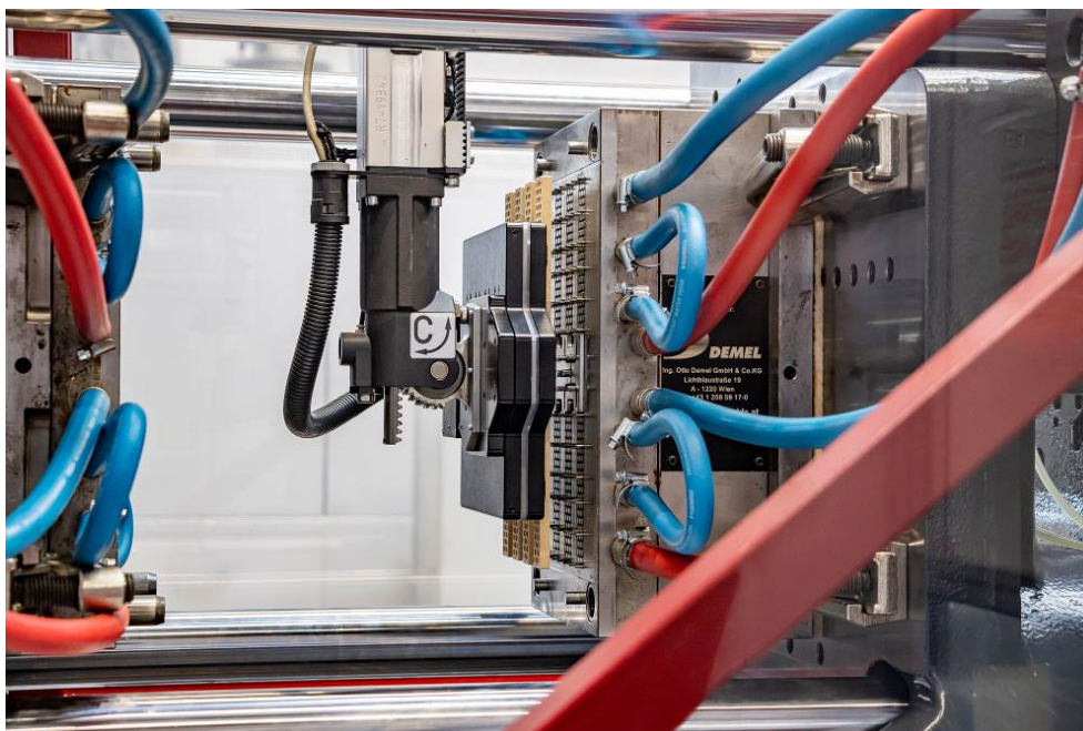
Fig. 2: Parts removal with WITTMANN robot W918
