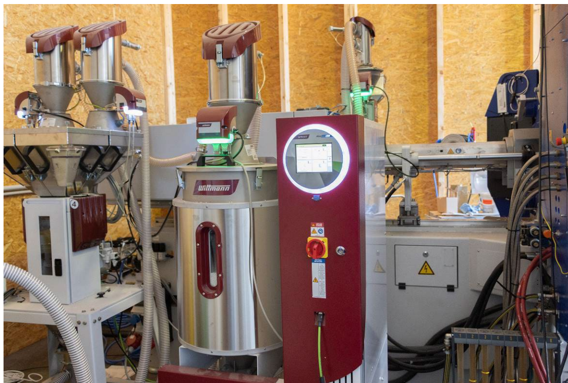
Fig. 2: Metering, material loading and drying technology from WITTMANN
