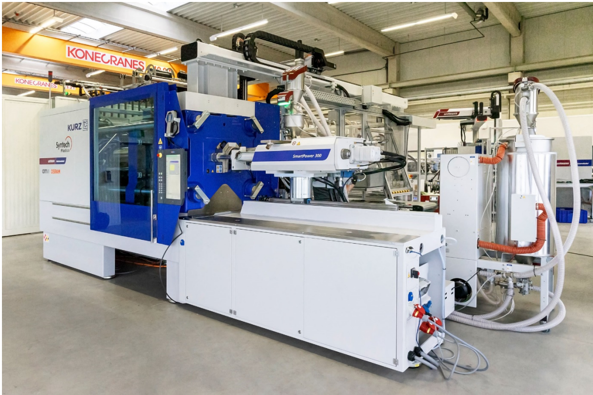
Fig. 1: Production cell for manufacturing parts with a decorated and functionalized surface
